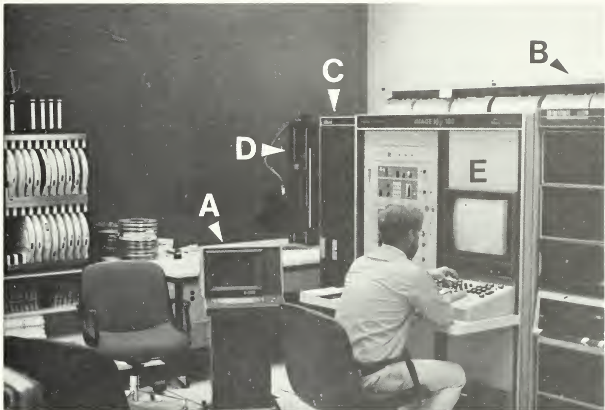
Figure 5 The Image-100 image analyzer consists of a control console and graphics display terminal (A) where commands are taken and returned by the system or where histograms can be displayed; magnetic tape drives (off the picture to the right); a PDP 11/35 computer (B); a solid-state memory module (C); an input scanner (D) and a video display unit (E) containing the image enhancement control panel. The analyst alternates his activity between the control console and image enhancement panel, as seen here. Analysts can learn to use the system effectively in a few hours.
