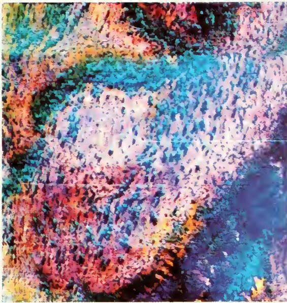
Figure 6 Color composites of Components 1, 4 and 5 displayed in blue, green and red respectively. Though colorful, the image fails to provide useful information on prehistoric sites.
