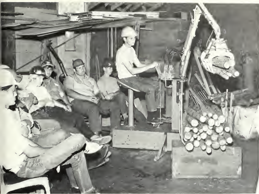
The Charlton County High School pulpwood class gets practical experience with the quarter-scale hydraulic loader. Coordination of foot and hand controls are a must. Built at a cost of $2,800, the loader is shared by 23 Georgia schools.
