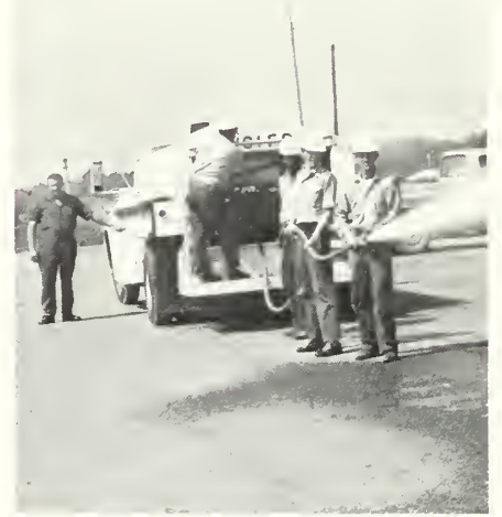
The 1,200 gallon capacity tanker is capable of pumping water at the rate of 125 gallons per minute.
