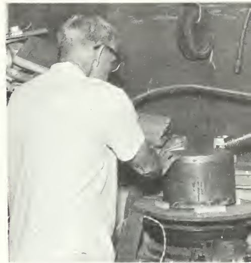
The finishing touches are put on the tube part of the oven. The homemade crimper consists of an automobile wheel and bearing and lawnmower bearing.
