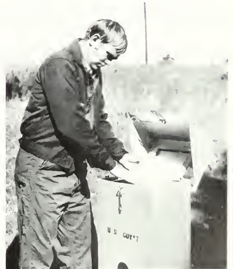
Spencer McGraw, ranger, Haralson-Polk Forestry Unit, inserts filter paper which traps particles in the air.
