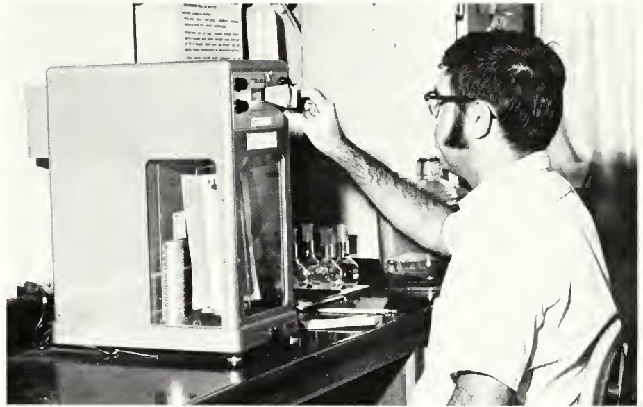
The difference in weight before and after sampling gives the weight of particles per volume of air. Darold E. Ward, research forester, USFS, conducts the testing.
