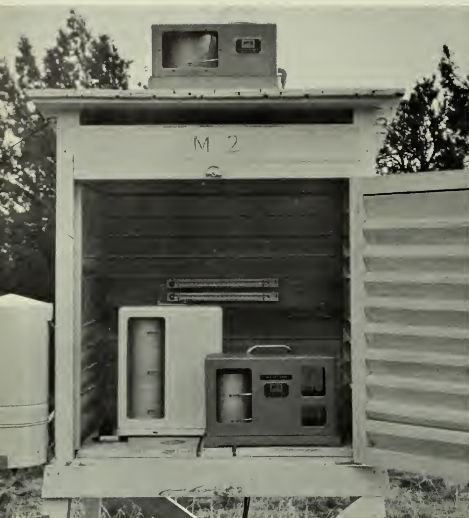
2 Recording instruments at M-2. Within the shelter are a hygrothermograph, a 3-pen mercury thermometer, and maximum-minimum thermometers. On the roof is a pyrheliometer, and mounted on the side is an atmograph.
