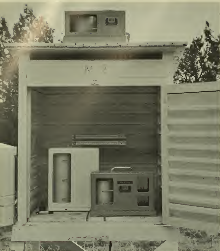
2 Recording instruments at M-2. Within the shelter are a hygrothermograph, a 3-pen mercury thermograph, and maximum-minimum thermometers. On the roof is a pyrliometer, and mounted on the side is an atmograph.
