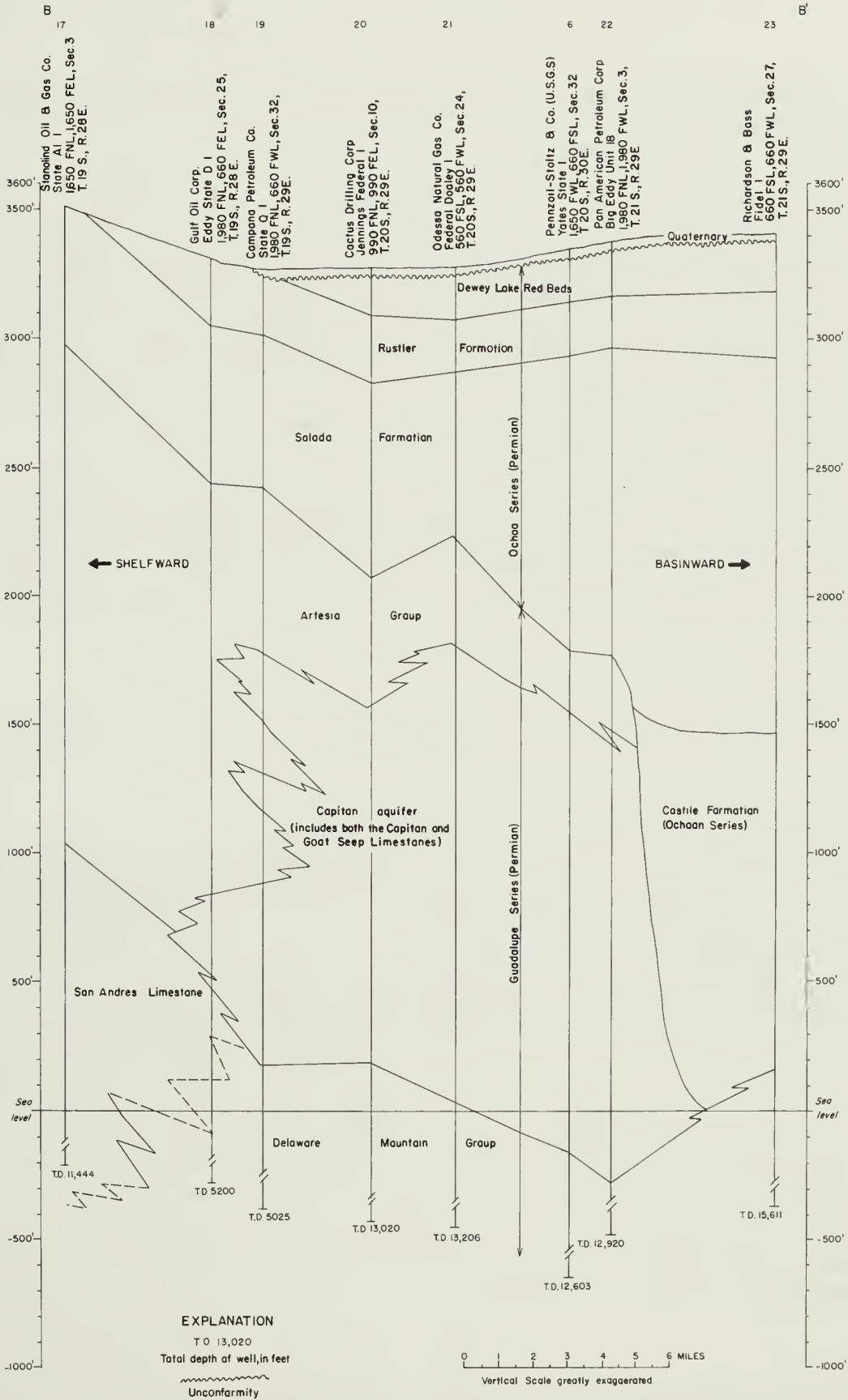
Figure 4.--Transverse stratigraphic section B-B' showing the position of the Capitan aquifer, Eddy County, New Mexico.
