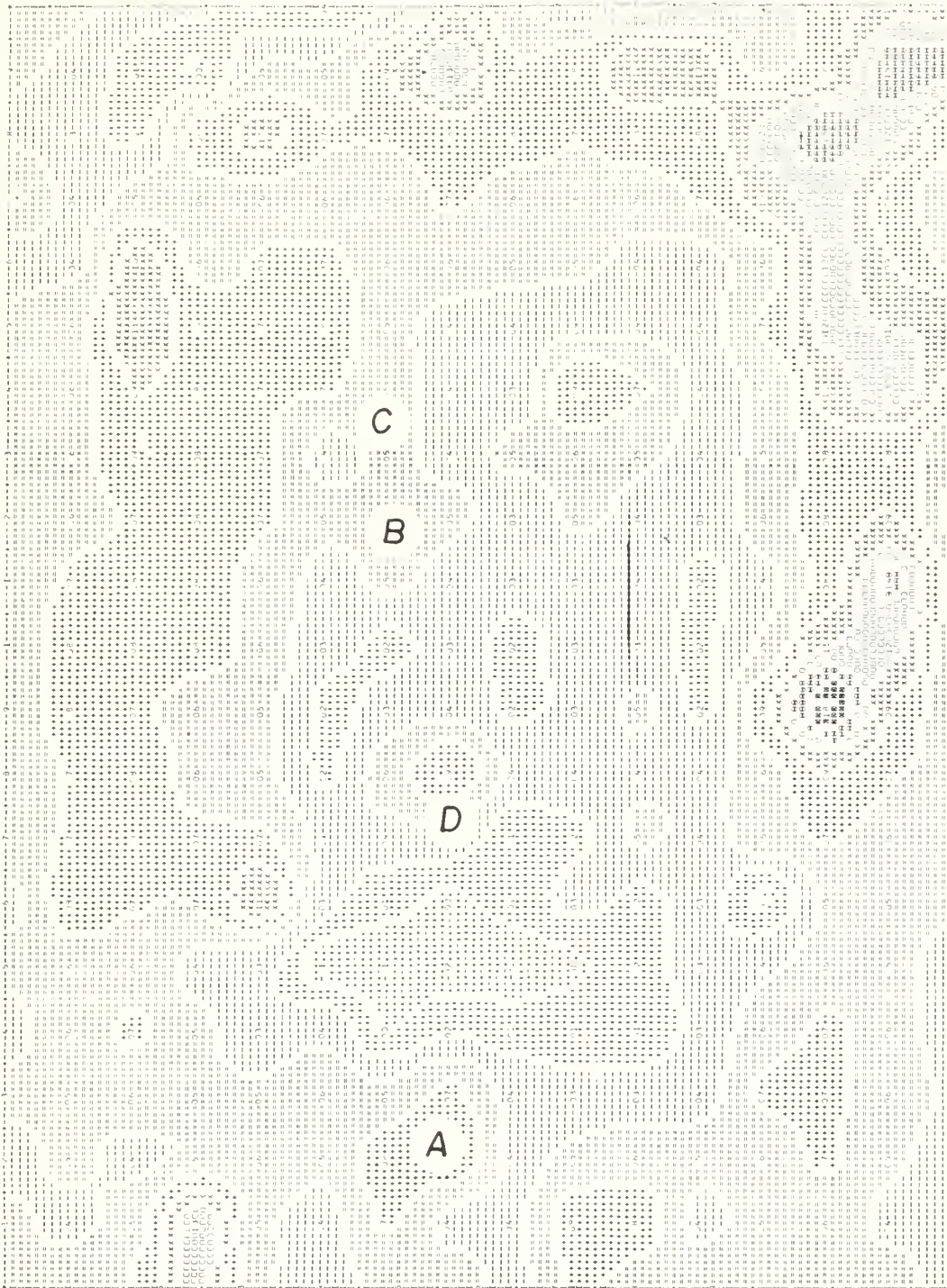
Figure 25. Magnetic map of House 19, Huff Site, North Dakota, produced by Harvard University's SYMAP program. Contour interval is 2.2 gamma. Courtesy of John W. Weymouth.
