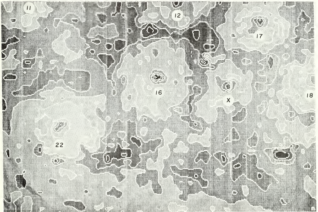
Figure 28. Magnetic map, Sakakawea Site, North Dakota; the block measures 40 by 60 m. Six earth lodges are visible on the surface in this area (Houses 11-22; house numbers directly below the central hearth of each house). One house (X) has no surface expression. Block location is shown in Figure 19. Courtesy of John W. Weymouth and the Midwest Archeological Center.
