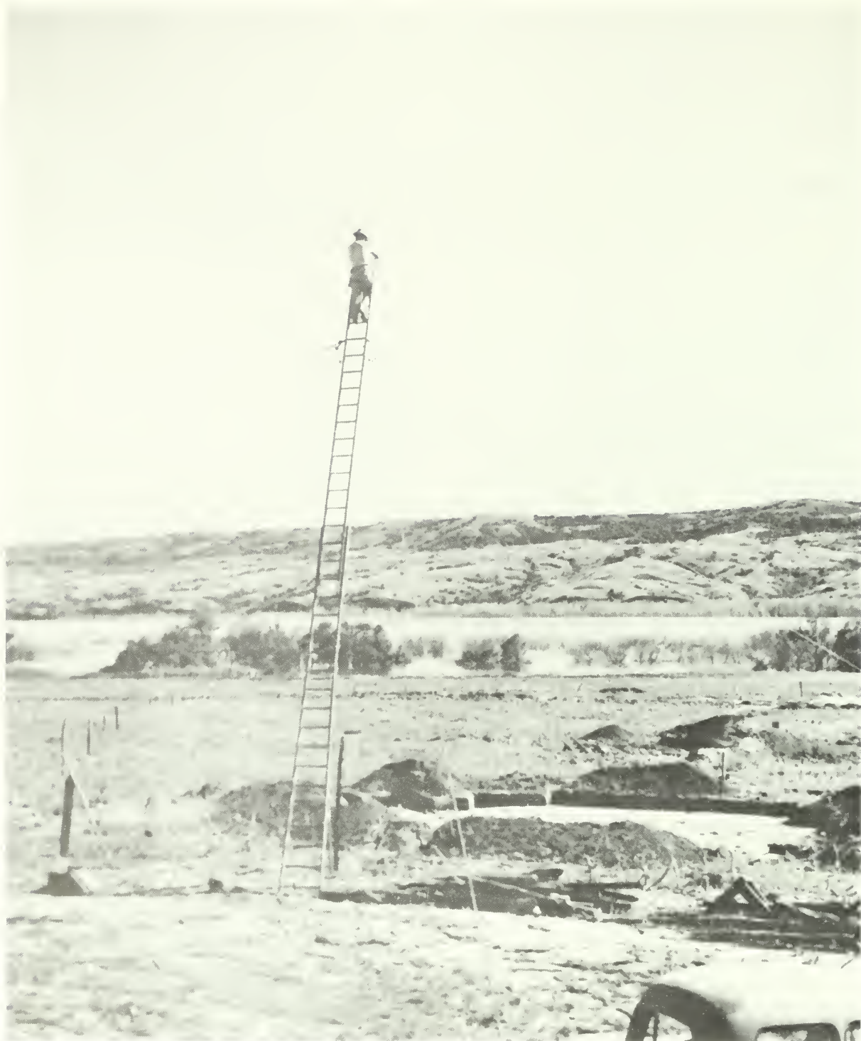
Figure 15. A low altitude ladder platform for oblique or vertical views, a once familiar sight on the Plains. Photograph courtesy of the National Park Service.
