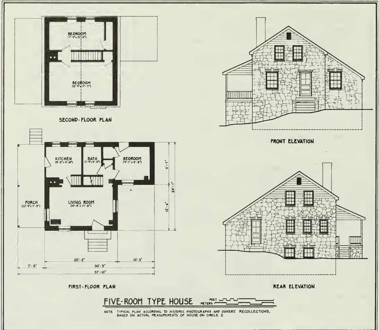
Figure 7 Plans and elevations of five-room house with front gable, shed-roofed ell. Delineator: Isabel C. Yang, HABS.
