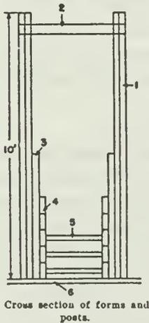
1. *Form post*: Made of 2—2 x 4—10 spiked or bolted together with  $\frac{1}{2}$ " iron pin fastened in bottom end, extending through bottom cross board #6.
