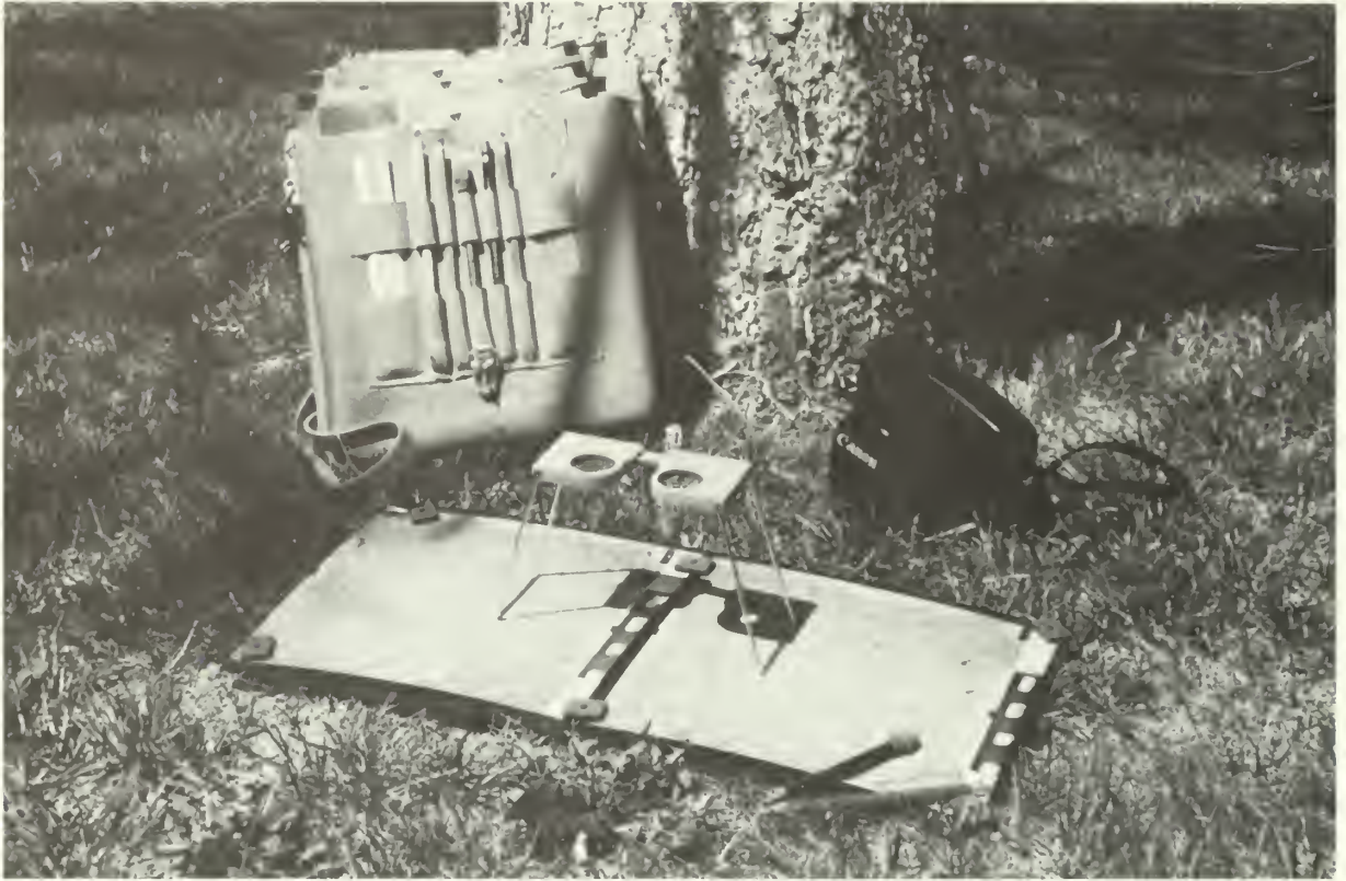
6-5 Portable kit for interpreting aerial photographs in the field.
