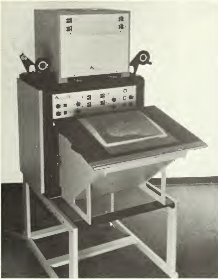
6-6 A multiadditive viewer for analysis of multiband imagery. Courtesy International Imaging Systems.
