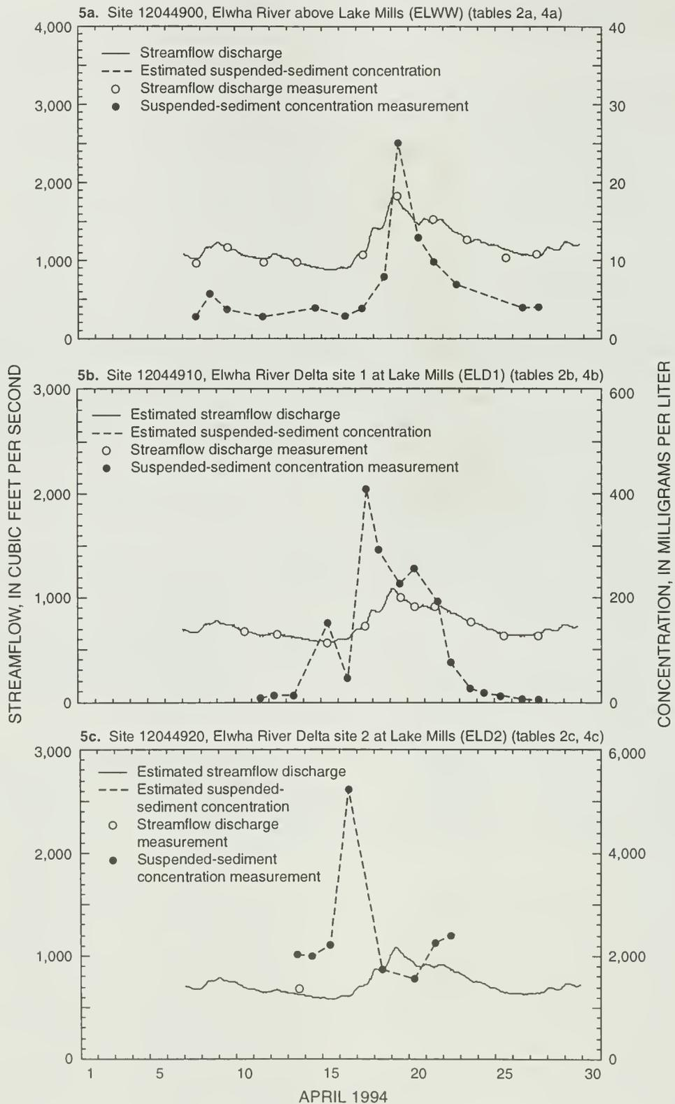
**Figure 5a-c.** Continuous record of streamflow and suspended-sediment concentration, instantaneous measurements of streamflow, and suspended-sediment samples at sites on the Elwha River, Washington. Whenever two consecutive samples were collected on the same day at a site, the average suspended-sediment concentration of the two samples is plotted.
