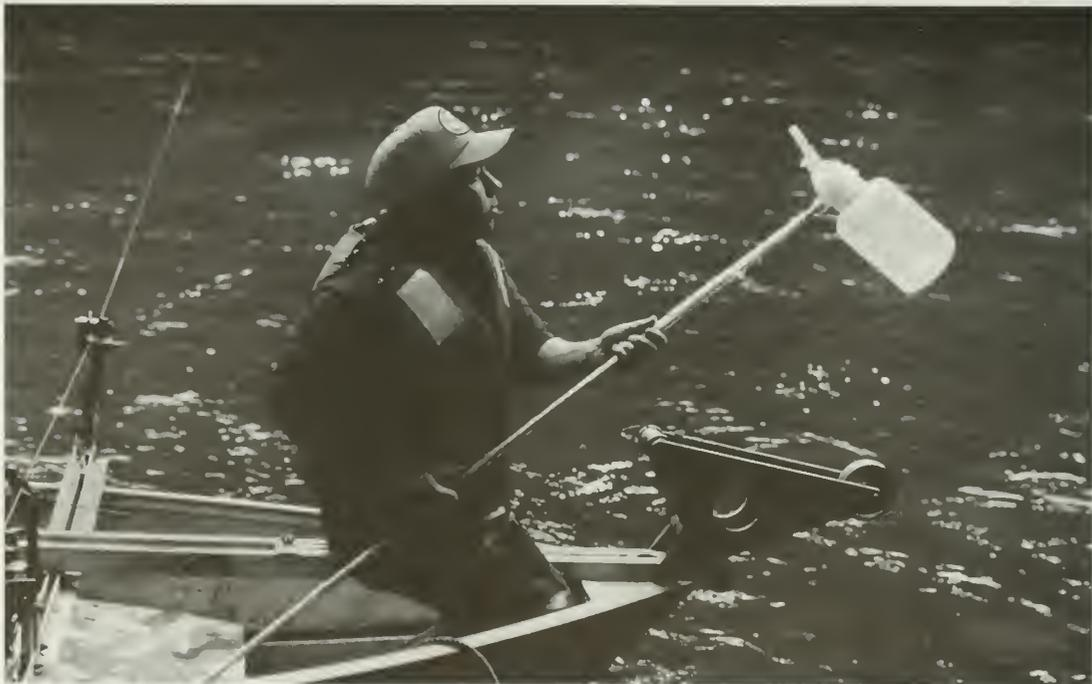
Figure 11. Wading-rod-mounted DH-81 water-quality and suspended-sediment sampler.
