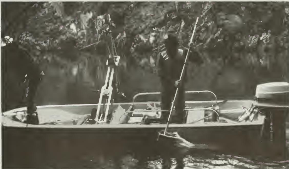
**Figure 7.** Sampling bedload at site 12044900, Elwha River above Lake Mills (ELWW), from a boat using a tether line attached to the boat gunnel.
