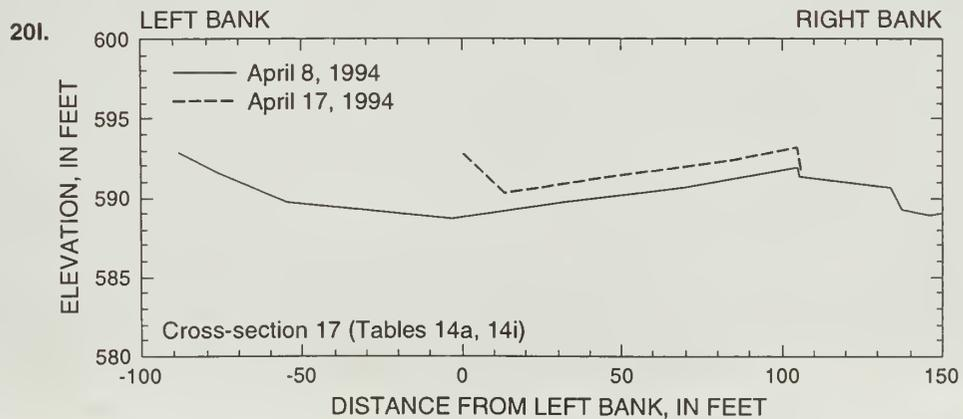
Figure 20i-l. Surface elevation of Lake Mills Delta, cross-sections 14-17.
