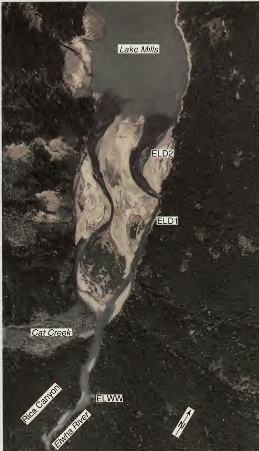
**Figure 3b.** Locations of streamflow and sediment data-collection sites ELWW, ELD1, and ELD2. Aerial photograph was taken on April 16, 1994, at time of full 18-foot drawdown of Lake Mills. Elwha River is flowing from south to north and has divided into a right (east) channel and a left (west) channel in the delta area. Photograph provided by the Bureau of Reclamation.
