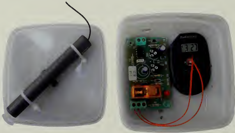
Figure 4. Example of a voice stamp assembly. The voice clock (far right) and timer/relay are secured in a plastic food container and the microphone is mounted to the lid. Enclosing the assembly in its own container helps isolate the microphone from the sound of the tape recorder running.
