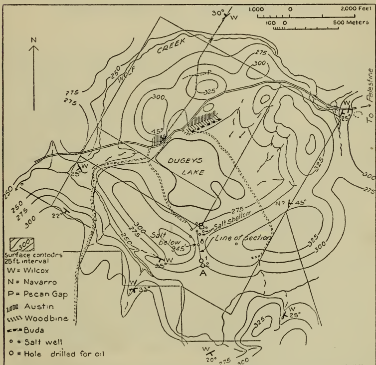
FIGURE 24.—Geologic and topographic map of the Palestine salt dome, Anderson County, Texas. For section along line A-B see Plate 12
