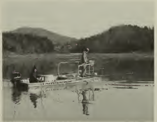
Electro-fishing boat used to obtain samples of fish. A generator charges the metal probes hanging from the poles at the bow of the boat, and the electrical current passing between them momentarily stuns the fishes nearby. (National Reservoir Research Program photo)
