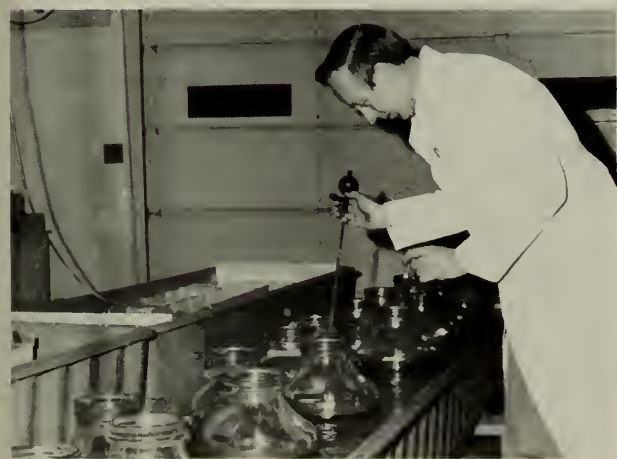
Adding a stock solution of the fish toxicant, antimycin, to static bioassay jars containing Asiatic clams. (Fish Control Laboratories photo)
