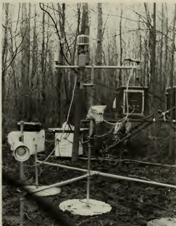
Micrometeorological studies are made in blackbird-starling roosts, which may contain millions of birds, to determine how weather can affect the success of roost treatments for control. Temperature and humidity were almost the same inside and outside the roost, but wind velocity was much reduced inside. (Photo by William J. Francis)
