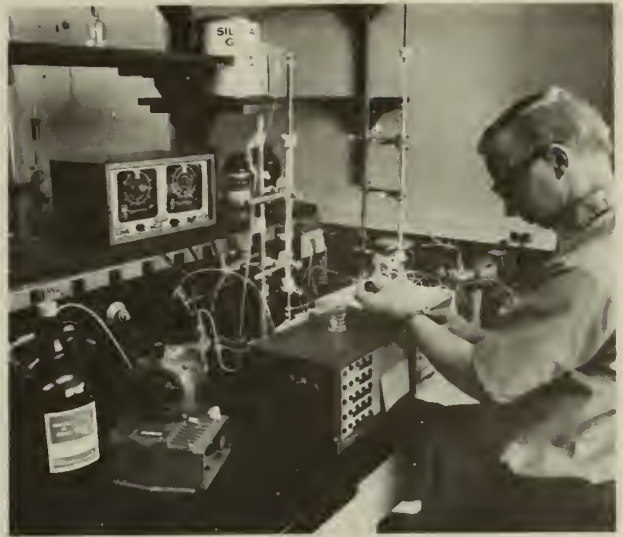
Preparing extracts of fish for pesticide analysis. The automated gel permeation system shown in use removes interfering fats and oils from extracts prior to gas chromatographic analysis. Samples are from fish collected in the Great Lakes to determine trends in pesticide residues, and from fish exposed to pesticides in the laboratory to evaluate the uptake and effects of various compounds. (Great Lakes Fishery Laboratory photo)
