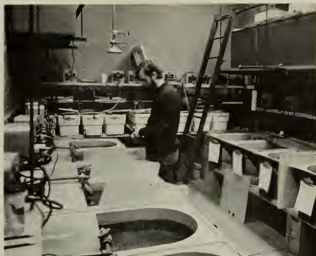
Feeding young lake whitefish in a laboratory experiment to determine the effect of water temperature on growth. Water is maintained at the desired temperature range in large overhead tanks and then adjusted to the desired precise temperature with thermostats and immersion heaters in each fish tank. The experiment is one phase of a broad study of energy flow in food chains of the Great Lakes. (Great Lakes Fishery Laboratory photo)
