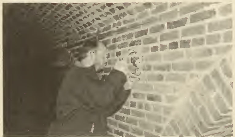
Pendulum hammer in use at Benjamin Latrobe's Basilica of the Assumption, Baltimore, Maryland
