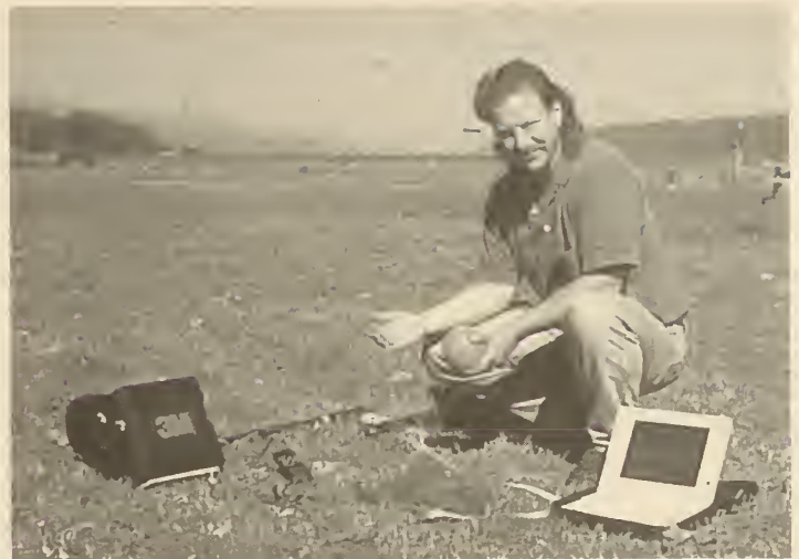
Washington State Parks archeologist Dan Meatt shown implanting an EMS marker. The device resting on the ground at left is an EMS transmitter.
