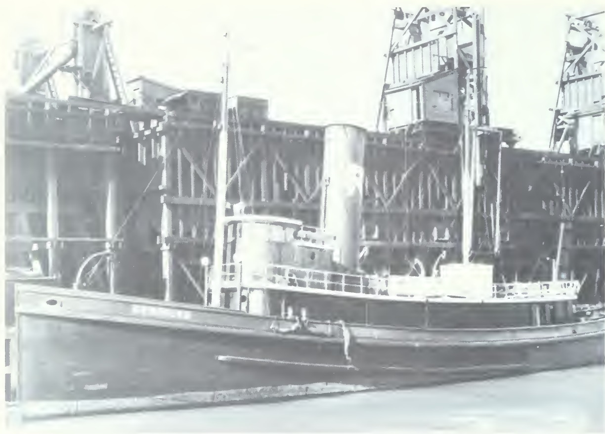
Fig. 5. HERCULES in the colors of the Rolph Coal and Navigation Company; black stack with large white "R." Note wireless shacks at mainmast, and antenna wires between masts.
