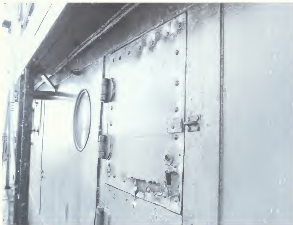
Fig. 21. Wastage typical of that seen in local areas of HERCULES' deckhouse.
