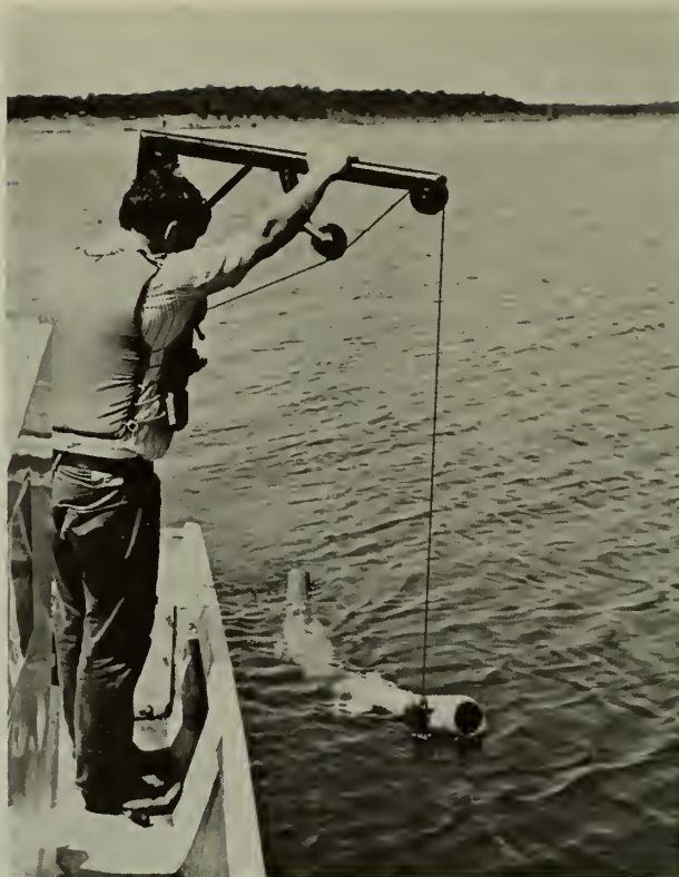
Retrieving a Miller sampler. Metered tow net samples are used to obtain estimates of seasonal zooplankton abundance on White River impoundments. (Photo by L. Barger)
