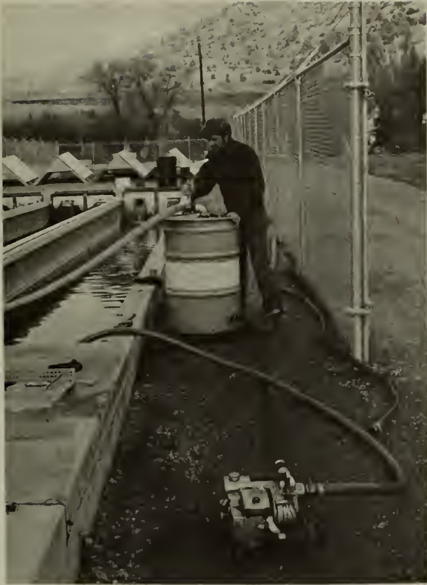
An experimental carbon filter system was effective for removing Furanace, a bactericide, from treated waters in trout raceways at the Fish Cultural Development Center, Bozeman, Mont. (Photo by L. L. Marking)
