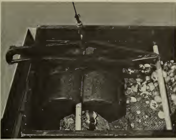
Organisms in the bottom of a body of water provide food for waterfowl. The organisms are sampled with this device, called a Petersen grab. (Photo by M. C. Perry)
