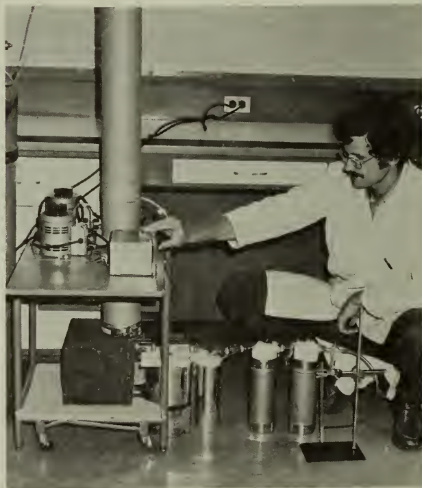
An apparatus used for the collection of rice volatiles. The "rice aroma" fraction collected in the apparatus is an excellent bait enhancer for Philippine ricefield rats. (Photo by Stanley Gaddis)
