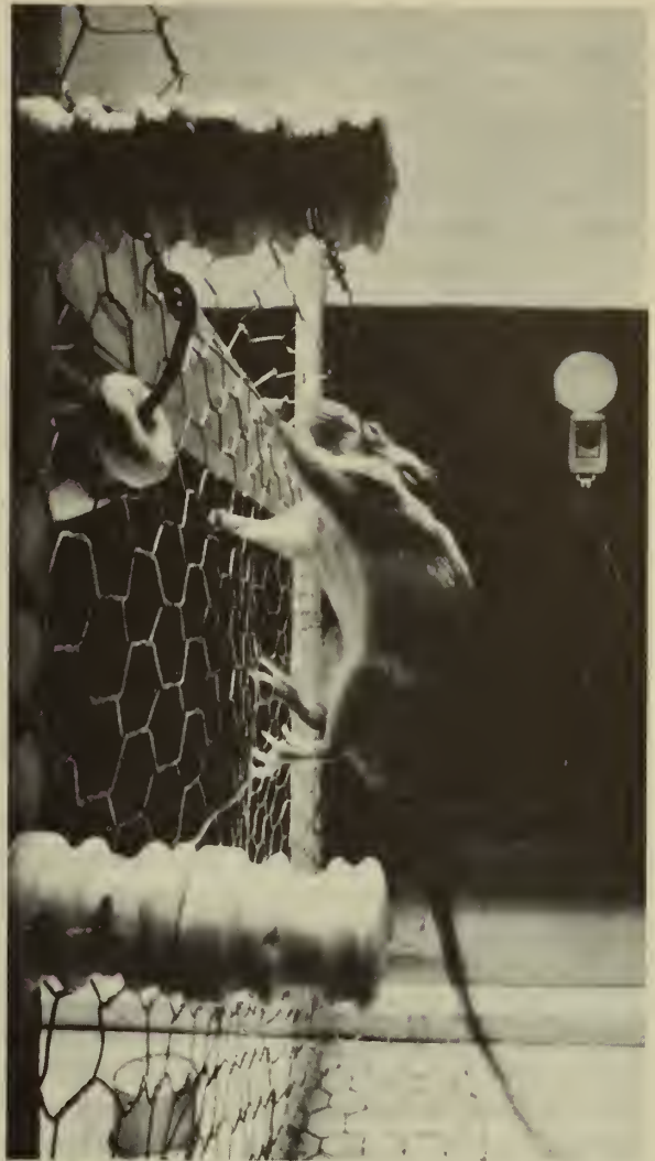
Ricefield rat attempting to climb a nonlethal electrical barrier in order to feed from a small container of rice. Detailed behavioral analyses of the rat-climbing activity is monitored through a closed-circuit television camera in the foreground. A 95% level of crop protection was observed with this barrier design in a field test in the Philippines. Photo by J. Stanfield, National Geographic Magazine .
