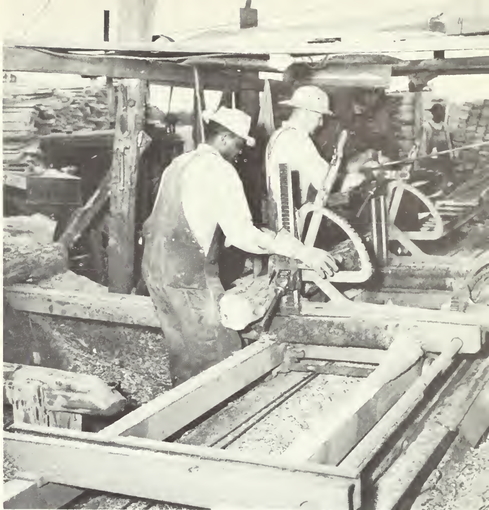
Buck Golden, sawyer, slices logs into seven foot box boards in the sawmill in top photo.
