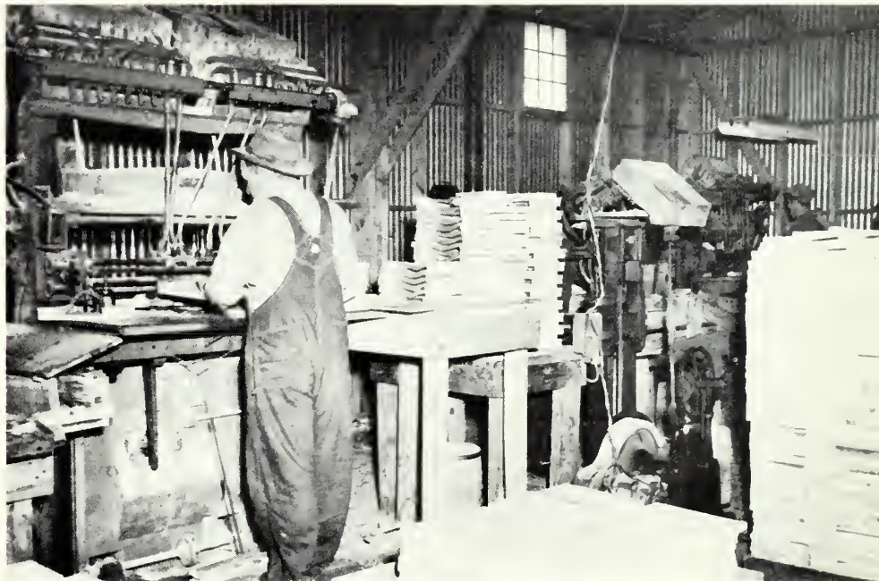
Boxes are assembled with a nailing machine (above). John R. Newman, Jr. (below) checks boxcar containing ammunition boxes ready
