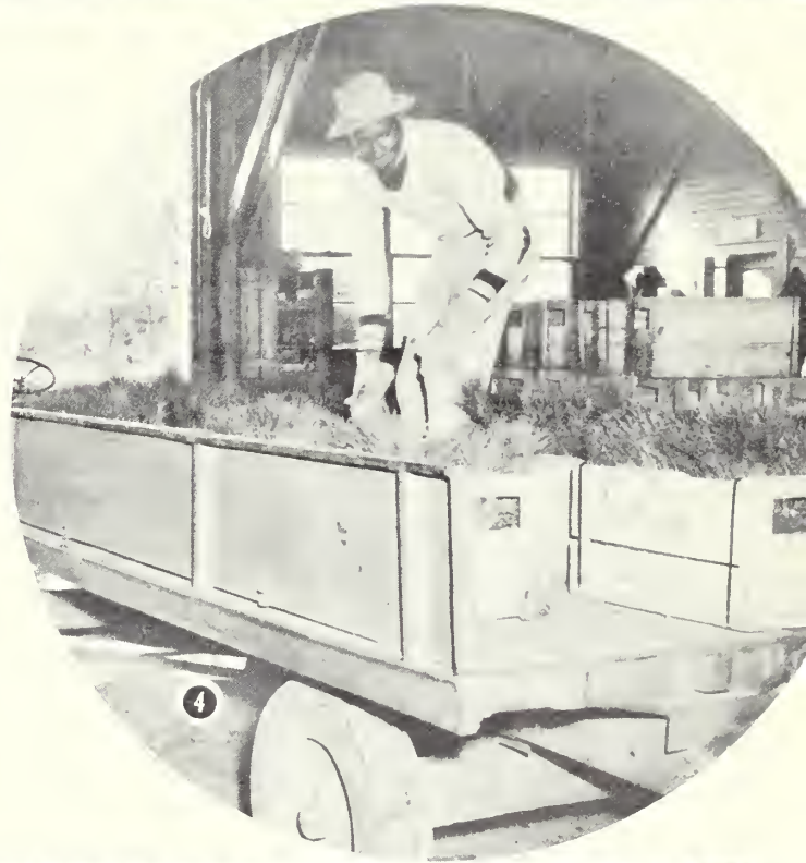
The tractor-powered seedling lifter, driven by Davisboro Nursery Superintendent Mack Neal, breaks ground under the seedlings, leaving them ready for quick hand gathering.
