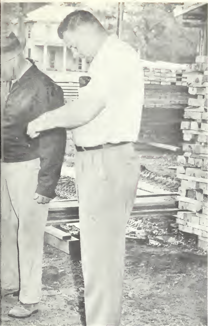
Moisture meter tells amount of water in lumber
