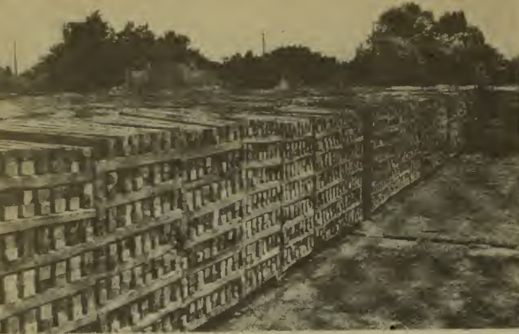
CROSS TIES stacked for seasoning at the East Point plant of Atlanta's Southern Wood Preserving Company.
