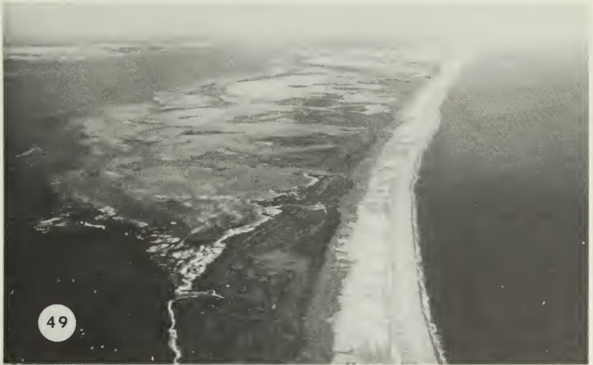
Fig. 49. Aerial view up Core Banks just north of the Cape Lookout Lighthouse, showing the uniform width (about 150 m) of the berm on this undeveloped beach. The width is set by major overwashes and their frequency. The light color along the back of Core Banks is ice, a rare occurrence in these waters. Sand waves along the beach are visible near the top of the photograph. The dark gray (almost black) zone bordering the lighter gray in the center of the island is a dense shrubland, frequently found running between the salt marshes to the left and grassland and dunes to the right.
