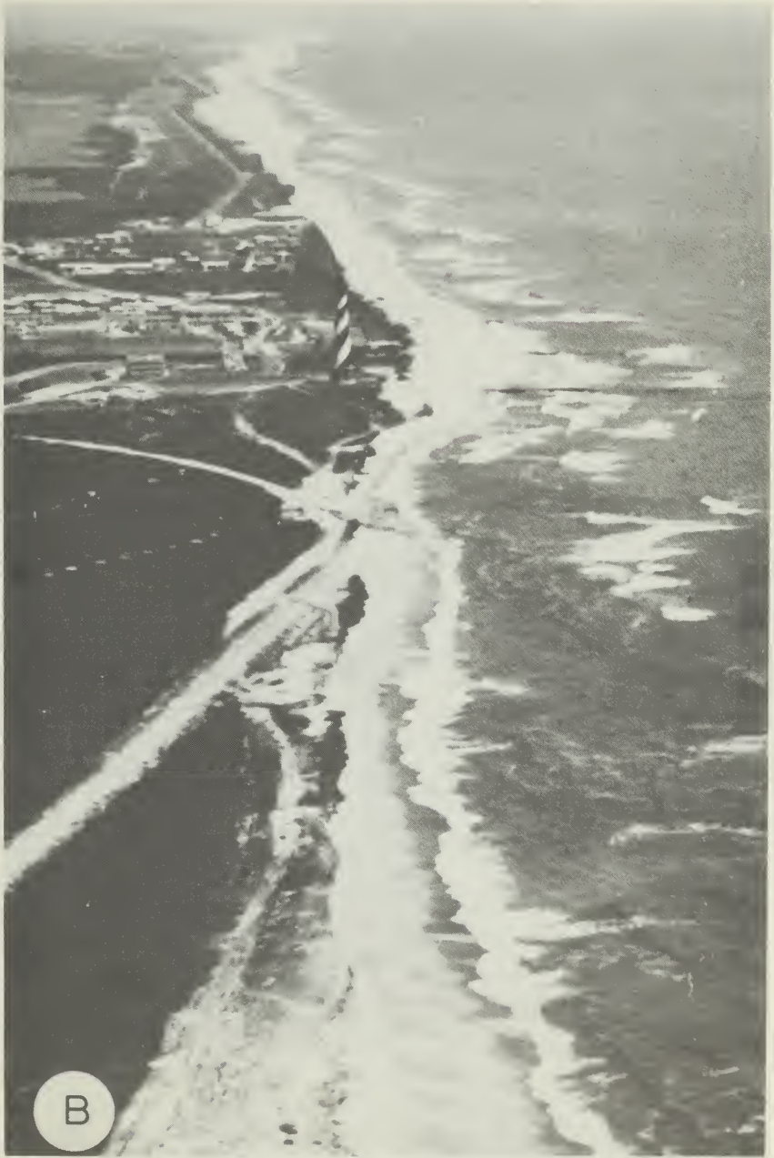
beach after groins were built in 1970. The groins have captured sand moving down the beach and the lighthouse is temporarily safe, but note how the artificial dune has been cut away by erosion on the downdrift side of the groin. ( Photo by Cape Hatteras National Seashore. )
