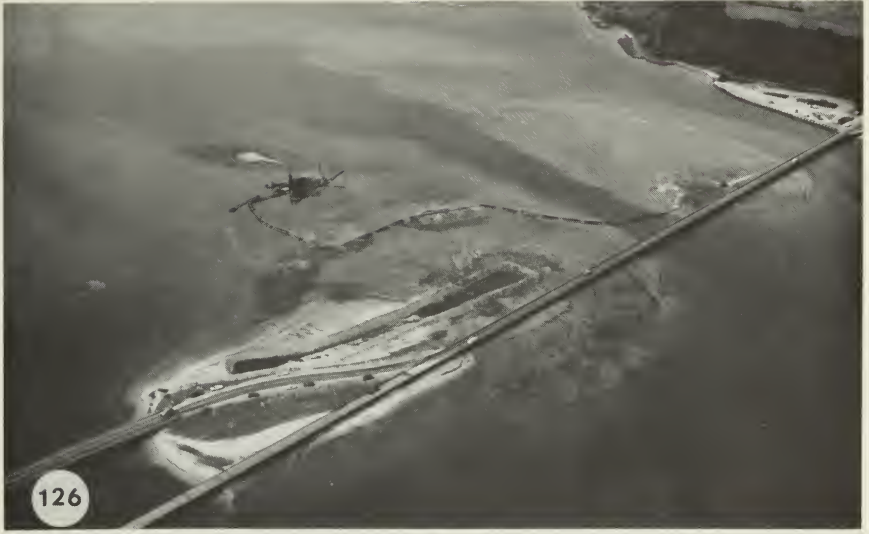
Fig. 126. A dredging operation in Carteret County, filling part of the estuary and making the rest turbid.
