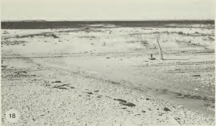
Fig. 18. Profile 14 on Core Banks, showing the bench marks established by the Corps of Engineers in 1960, and elevation changes. When constructed, the concrete base was at the level of the sand. Profile 14.0 in the foreground is now located in an overwash channel and shows some loss of sand from the base; 100 ft back is P 14.1, just visible in the photograph. Sand covers the base of this marker.
