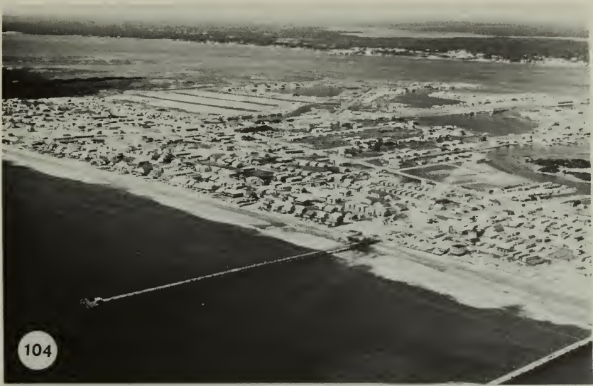
Fig. 104. Bogue Banks at Atlantic Beach. Marshes have been dredged and bays filled for housing developments and trailer parks. All are vulnerable to a big hurricane.
