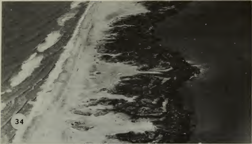
Fig. 34. The same part of Core Banks as shown in Fig. 29, after Hurricane Ginger. The photographs in Fig. 29 were taken opposite the number "34." Contrast this view with Fig. 32. On the undeveloped beach, overwash builds up the inner part of the island. Past overwash deposits are clearly visible in this view. The area is just south of the view of the Coast Guard Station in Fig. 23. In December 1971, the Corps of Engineers cut a new inlet through the narrow neck near the top of the photograph. (See Fig. 10D.)
