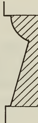
CARPENTRY SHOP DOOR PANEL MOLDING; main Barn side, Carpentry Shop side; 4 plain recessed panels
