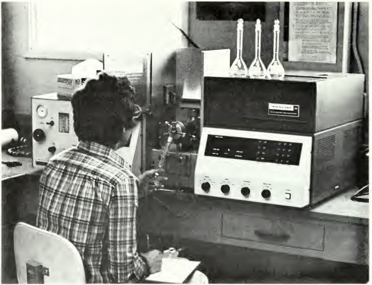
Chemist operating atomic absorption spectrophotometer as part of project to increase salmon returns by improving the health and quality of the smolts released. Photo by William T. Yasutake.
