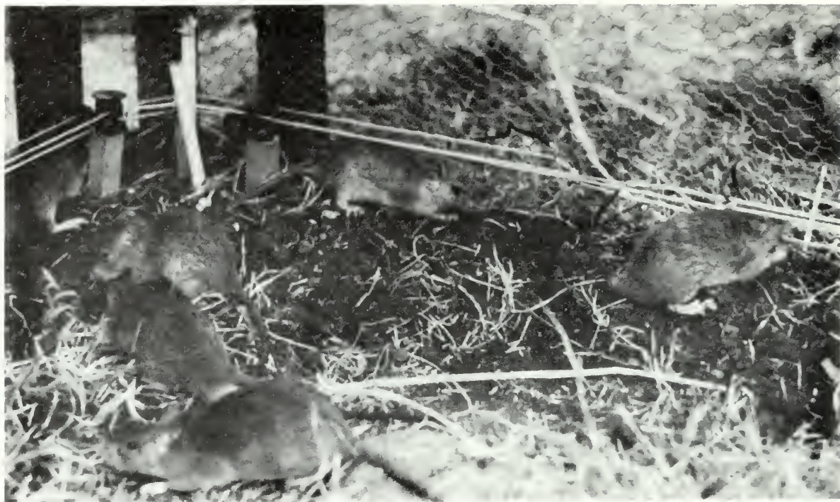
These six rice-field rats are trying to escape an enclosure having a 3-wire electrode system and a nonelectrified vertical barrier designed to prevent rats from invading rice fields. Photo by A. Lawrence Kolz.
