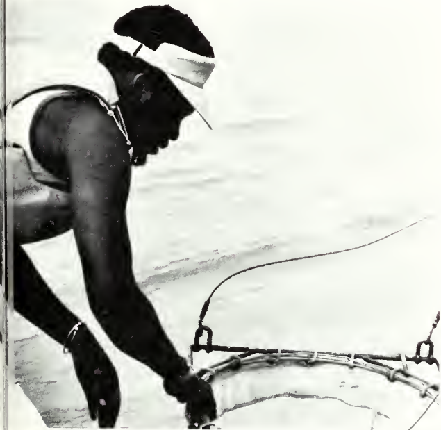
Sampling fish larvae with 0.5-m plankton net to determine locations of spawning and nursery areas in the St. Clair-Detroit River system. Photo by Roann Ogawa.
