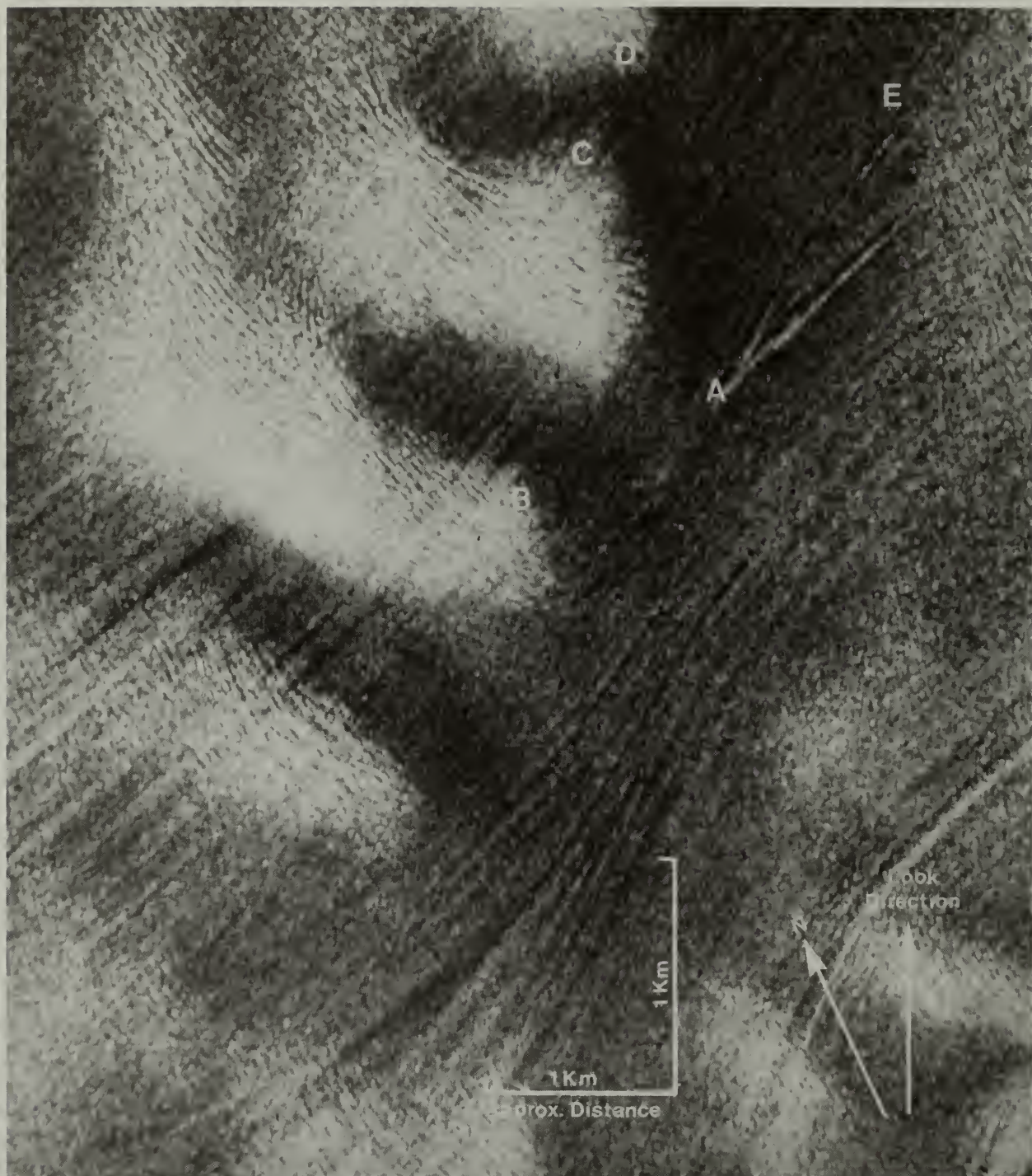
Fig. 2. An enlargement of the area outlined in the rectangle in Figure 1. The tip of the moraine (A) was the base station for a doppler geociever and served as the starting point for four planetable/alidade profiles across (A to B, C, and D) and along (A to E) the northeast trending swale. This swale, seen as a dark area on the image because of low radar backscatter, had a relief of more than 40 m. The four dark, elliptical, cirque-like patterns on the left flank of the swale are bounded by bright-return topographic highs. The swales are zones with few crevasses, while the highs are characterized by an extensive crevasse network. The scales parallel and perpendicular to the look direction are different due to SLAR imaging anomalies.
