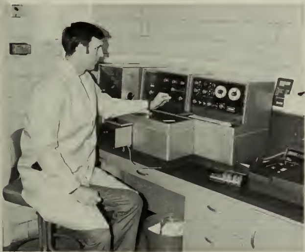
Spectrophotometer used to measure physiological effects of chemicals. Serum enzyme activities show tissue damage induced by organophosphates, organochlorines, or heavy metals. Enzyme effects, which are useful in both field and laboratory investigations, are being studied in many species. (Photo by John Maestrelli)
