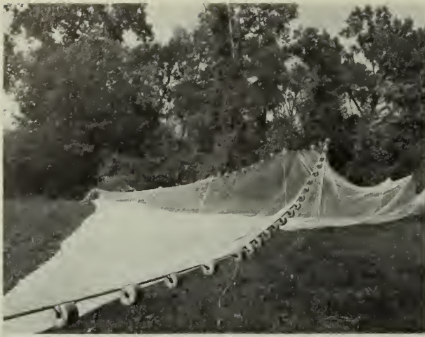
An experimental "scoop" net is being developed at the New York Cooperative Fishery Research Unit for obtaining large samples of small fish in ponds with minimum damage to the fish or their habitat.
