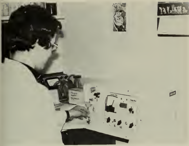
Electrometric titrator determines physiological changes in the blood of fish following stress. (Photo by D. E. Crouch)
