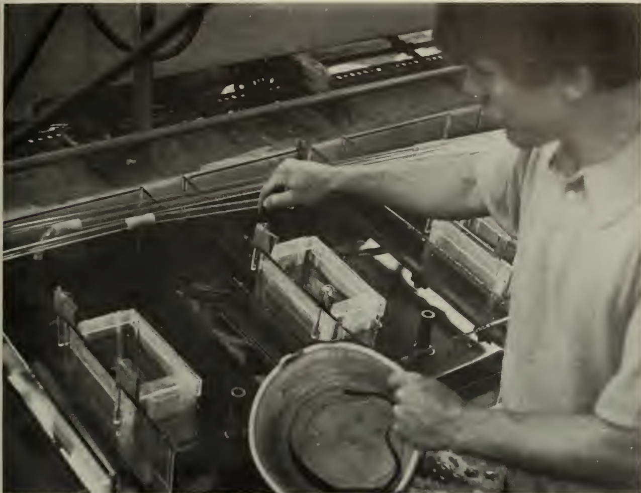
Larval sea lampreys are exposed to lampricides in flow-through tests which simulate natural streams. (Photo by Leif L. Marking)
