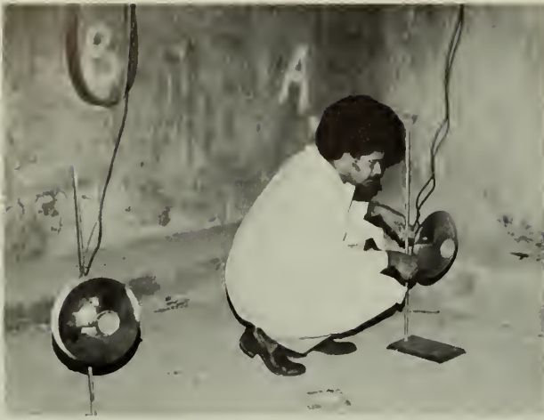
In simulated warehouse tests, a biologist evaluates ultrasonic devices claimed to repel rodents. (Photo by G. Keith LaVoie)
