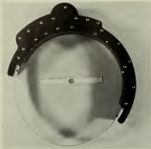
This 4-pound transmitter for grizzly bears functions as a normal, fast-pulsed radio-tracking unit while the animal is active but switches to a slow pulse during hibernation to conserve the batteries. (Photo by A. Lawrence Kolz)
