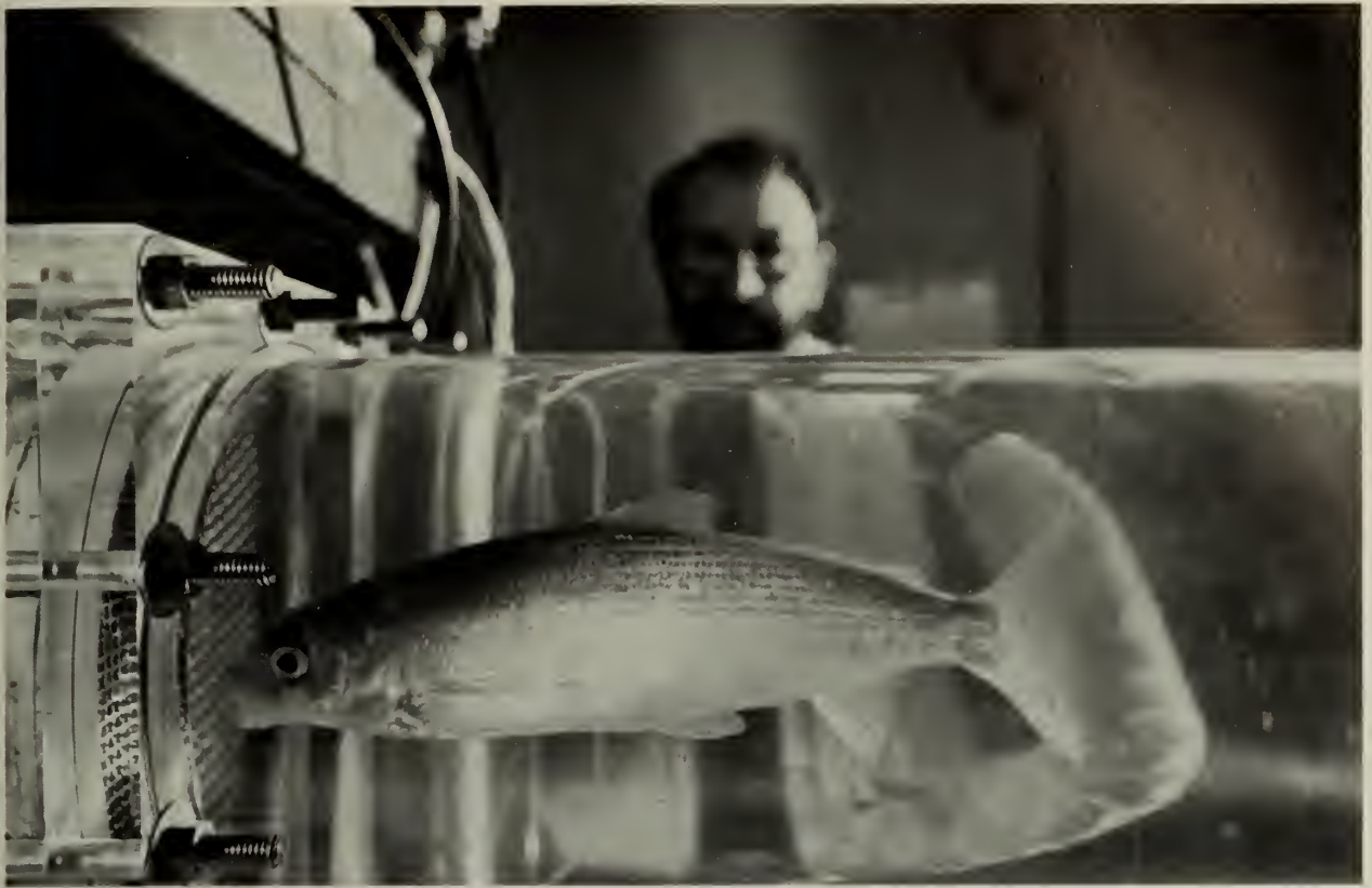
Measuring the oxygen consumption of a lake whitefish during forced swimming in a tunnel respirometer. (Photo by Thomas Ramsey)
