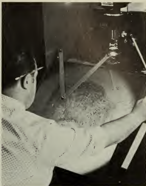
Determining the age of a fish by projecting the magnified image of its scale. Because annual growth of the scale is proportional to the growth of the fish, the length of the fish at the end of each year of life can be calculated and its growth history reconstructed. (Photo by Robert Reinert)
