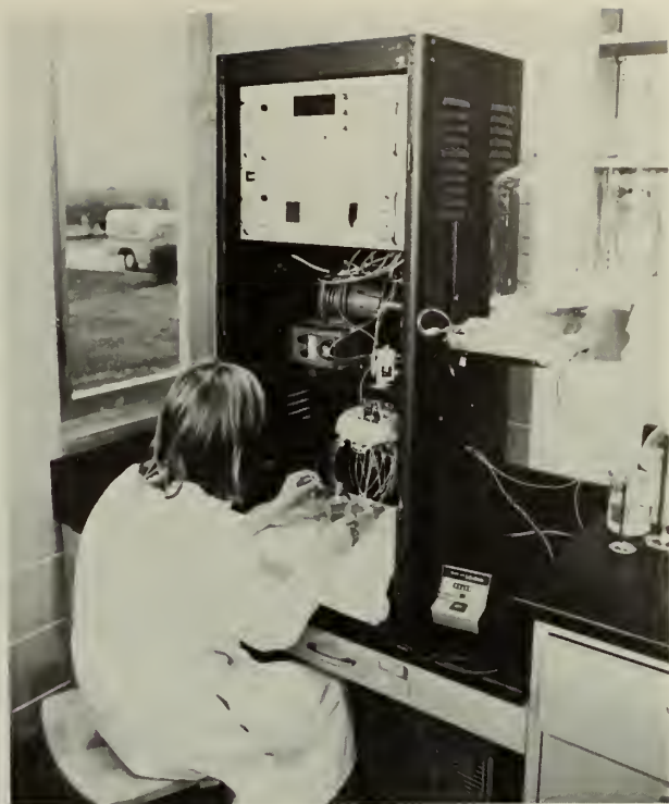
Automated gel permeation chromatography unit developed at the Fish-Pesticide Research Laboratory for separation of lipids and pesticides.
