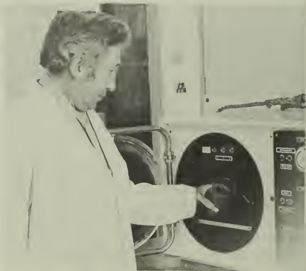
Freeze drying in a lyophilizer is the final step in preparation of Hagerman red-mouth vaccine. (Photo by D. E. Crouch)
