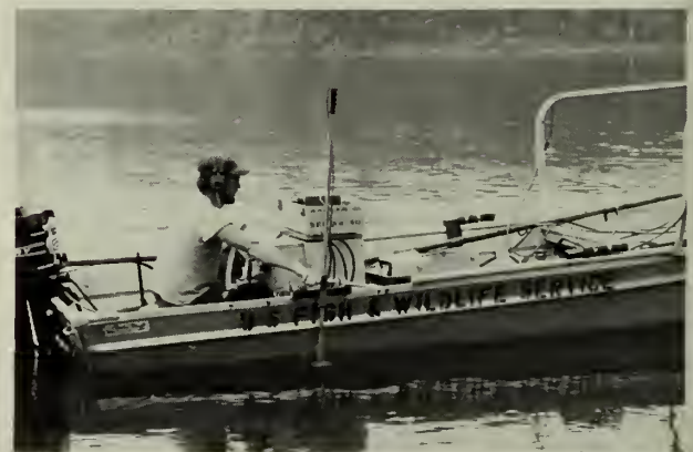
Boat equipped with transducer, receiver, and earphones to pick up signals from the sonic tag.
