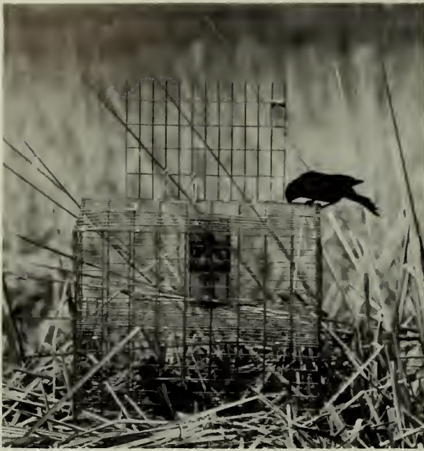
This new double-compartment trap has proved very effective in capturing territorial males for banding and color-marking in Wyoming and Colorado. This territorial male is about to enter the trap to attack the decoy, an adult male redwing in the lower compartment. (Photo by Olin E. Bray)
