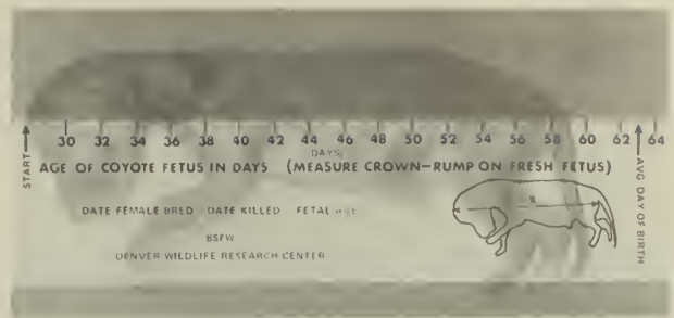
A ruler-like measuring device with superimposed 58-day-old coyote fetus. The ruler was designed for aging coyote fetuses and determining breeding dates in the field (actual size of ruler, 2 × 8 inches). (Photo by Brad E. Johns)
