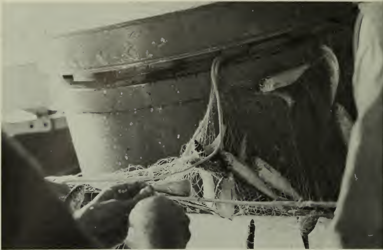
Alewives being removed from a portion of the gill net which has just been released from the jaws of a hydraulic gill net lifter. The net is pulled from the water through a window in the enclosed foredeck of the vessel, and passes around the head of the lifter in a clockwise direction. (Photo by LaRue Wells)
