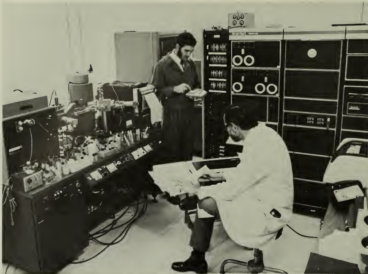
Computerized gas chromatograph-mass spectrometer in use at the Fish-Pesticide Research Laboratory.
