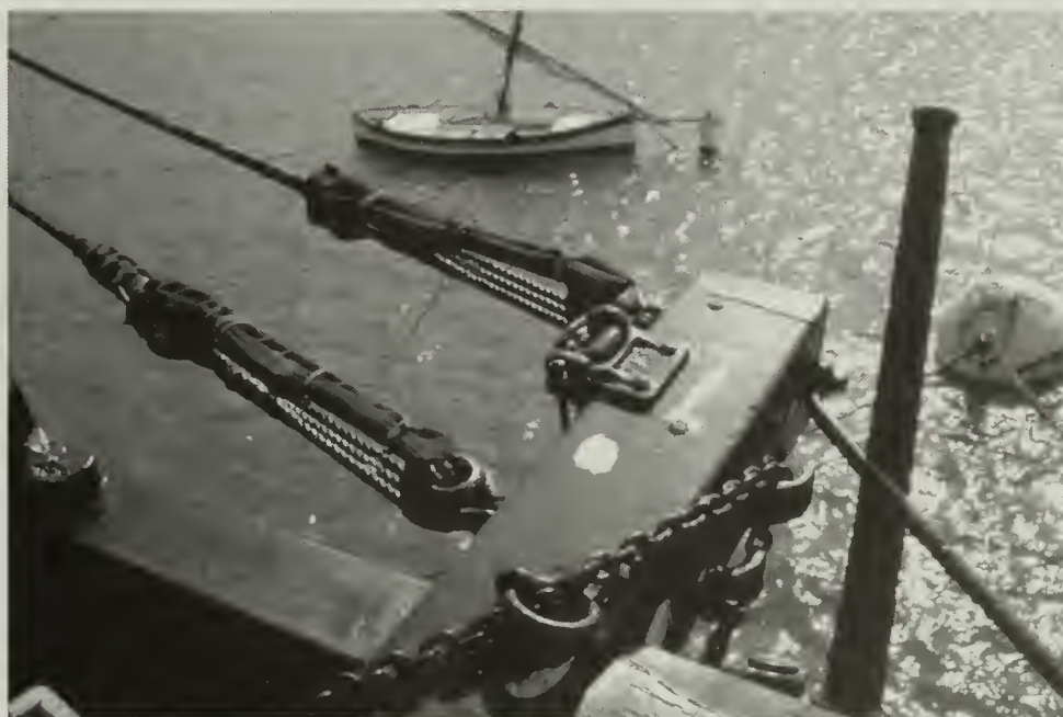
Figure 4.92. Rigging element supporting jibboom guys on forward side of C. A. Thayer ’s cathead. NPS photo by Matt Russell.
