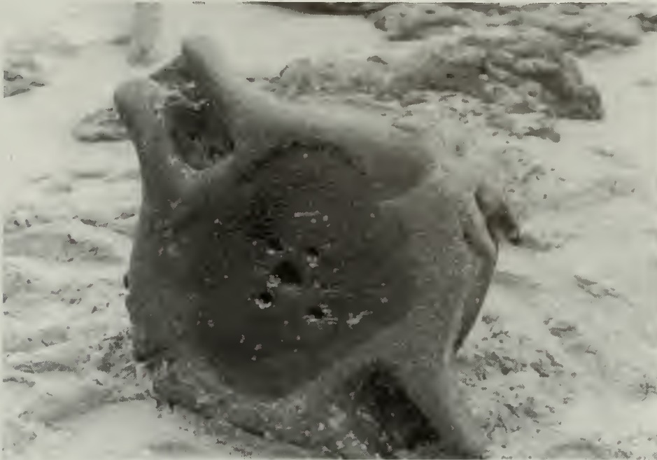
Figure 4.50. End view of the yoke attached to the end of a rudder stock. NPS photo by Don Morris.
