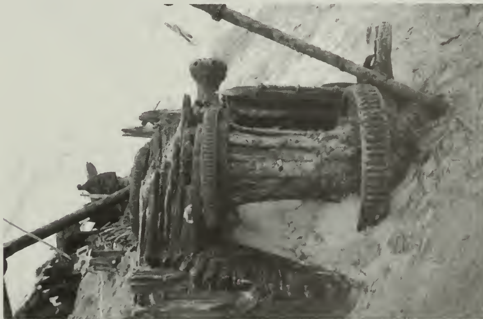
Figure 4.82. Photograph taken from the perspective as if the viewer were standing on the main deck looking forward. The pawl post is to the left of the windlass. NPS photo by Matt Russell.
