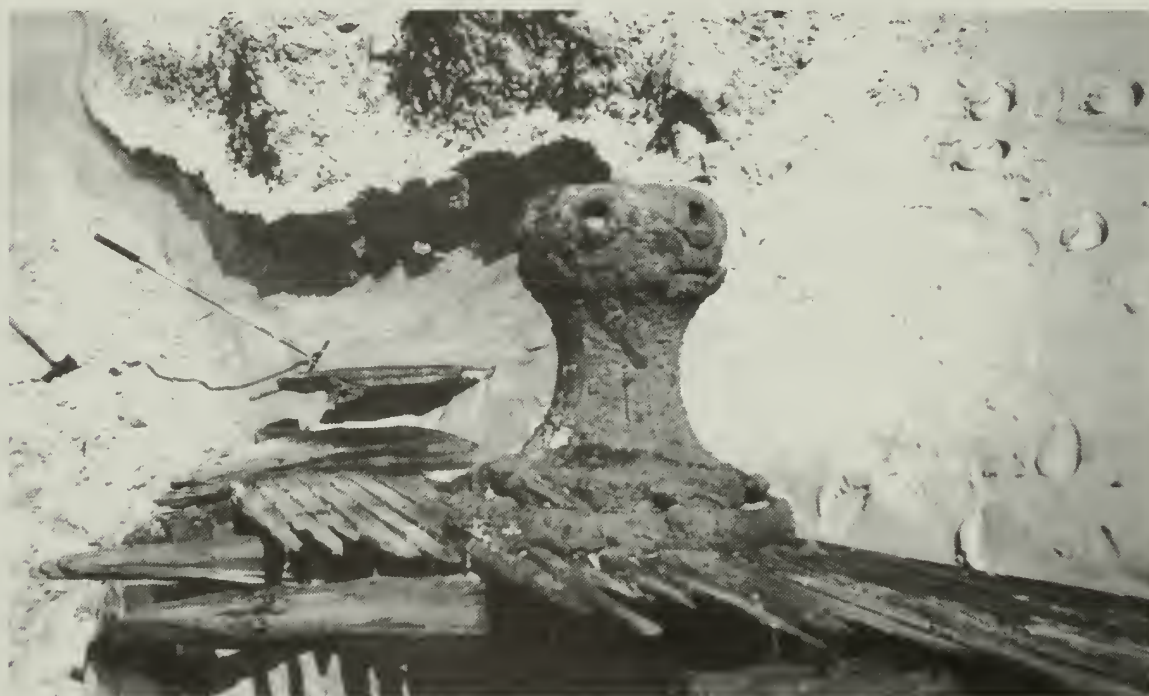
Figure 4.103. Comet's capstan, mounted in the center of the forecastle deck. NPS photo by Don Morris.
