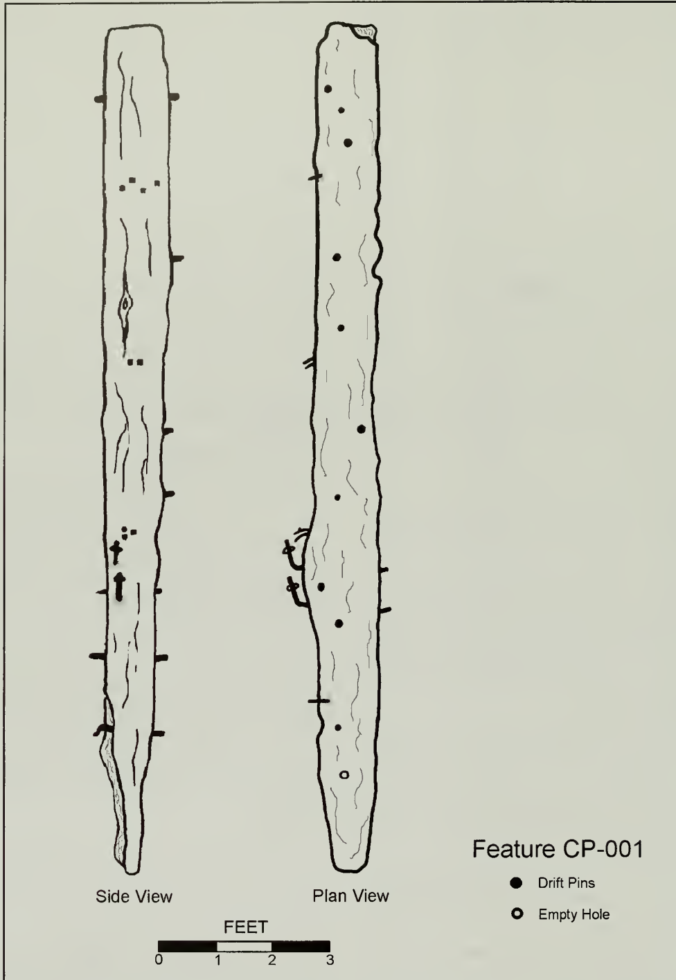
Figure 4.53. Keelson element with iron fasteners (feature CP-001). Drawing by Matt Russell.
