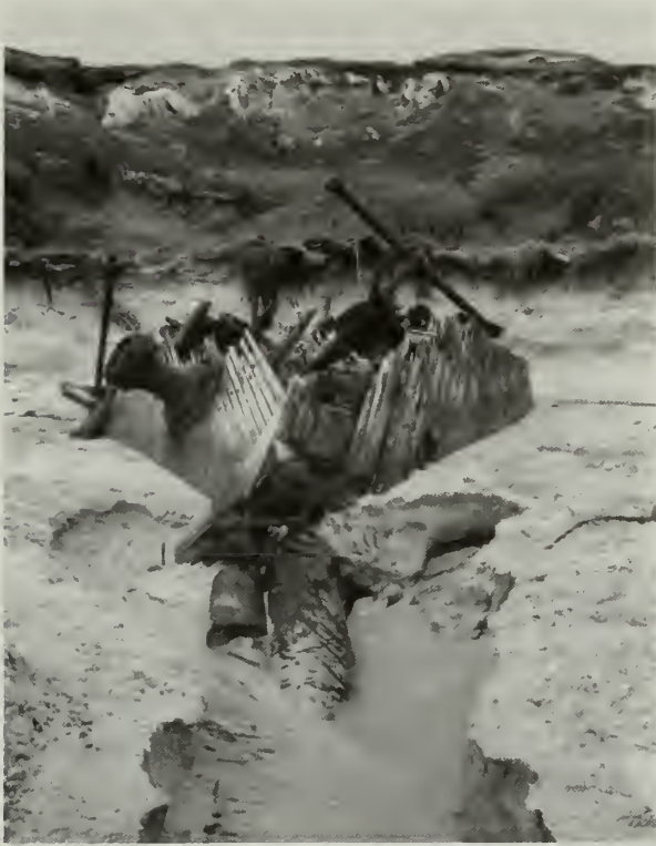
Figure 1.5. Comet site in April 1999, looking straight towards the bow, which is canted to the left in this photo. The forecastle deck is to the left, port side outer hull planking to the right and the bowsprit is in the bottom of the photo. NPS photo by Matt Russell.
