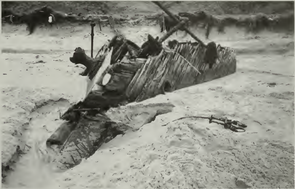
Figure 4.75. Comet's bow. The hawse timbers are in the center with the white float on them. The hawse pipe is visible at the sand-line, to the right of the hawse timbers. In the right foreground is an unattached rigging element. NPS photo by Matt Russell.
