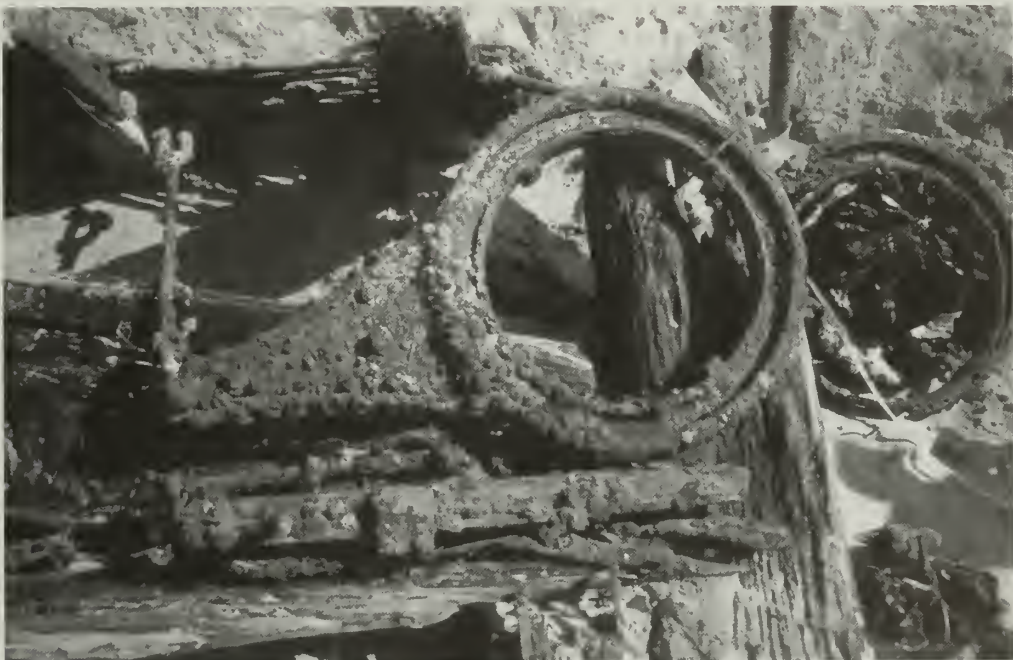
Figure 4.97. Comet 's port windlass purchase arm and windlass hardware on the main deck laying against the port side of the pawl post and bowsprit. NPS photo by Don Morris.
