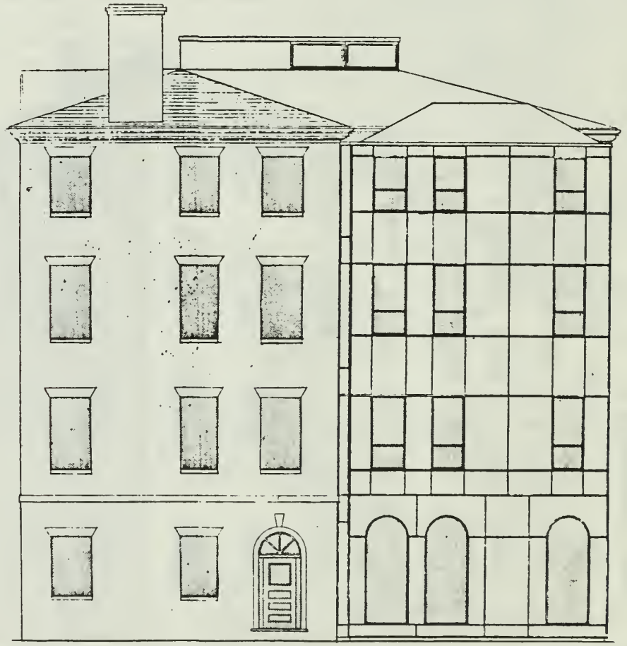
Illustration #4. ELEVATION The new 4 story addition visible from the street would be compatible in scale and proportion with the historic structure. The pattern of window and door openings in the new addition would reflect the rhythm in the historic facade. The use of a modern panel system, as opposed to detailed brickwork, would clearly separate the new construction from the historic resource. The use of a separate hipped roof for the addition would retain the scale of the property and would eliminate damage to the historic roof and cornice.
