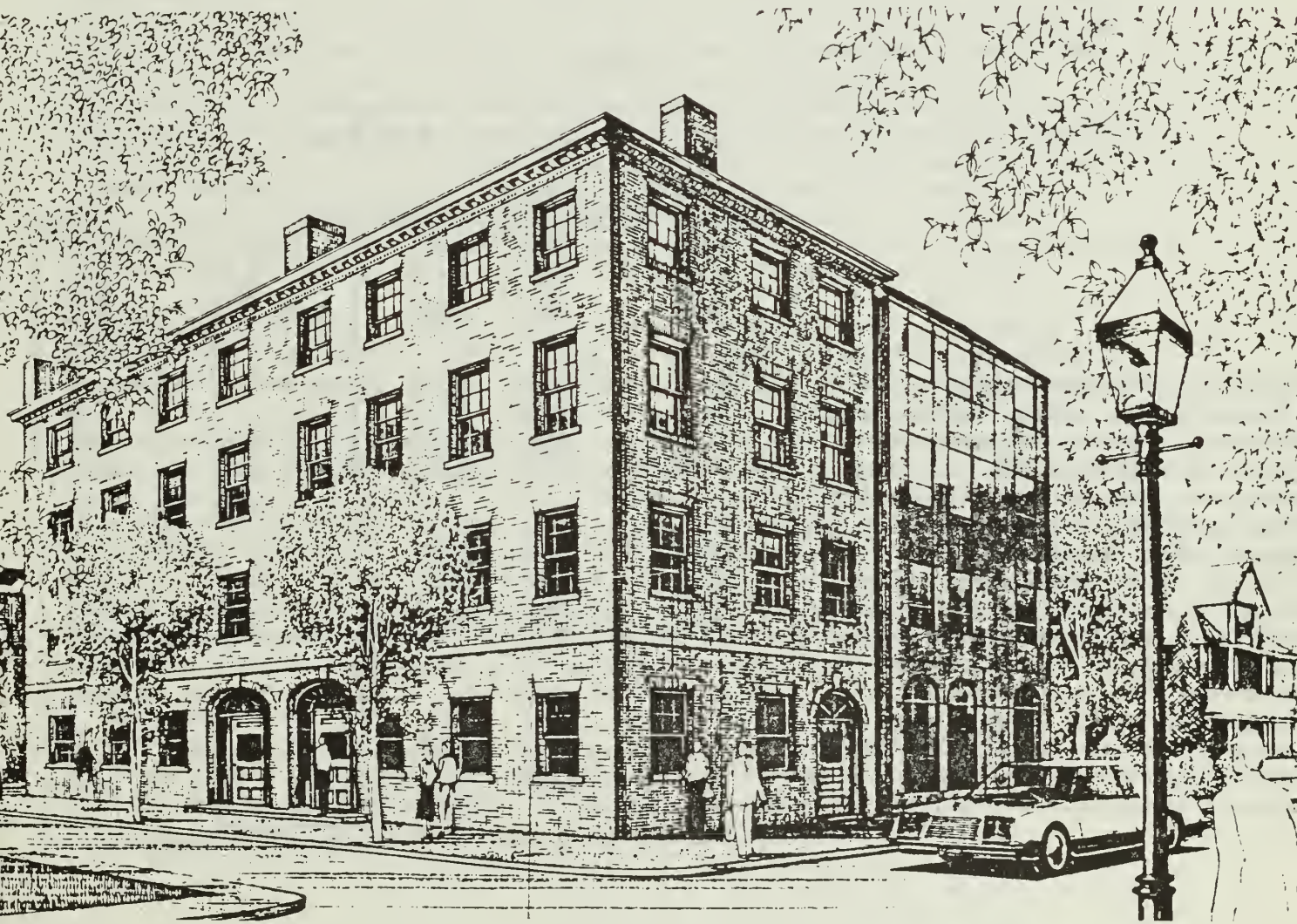
Illustration #2. PERSPECTIVE VIEW. The revised design treated the rear addition as a modern pavilion to clearly differentiate it from the historic structure.
