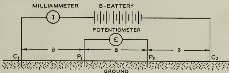
FIGURE 11.—Schematic diagram of the Wenner system for measuring earth resistivity.
