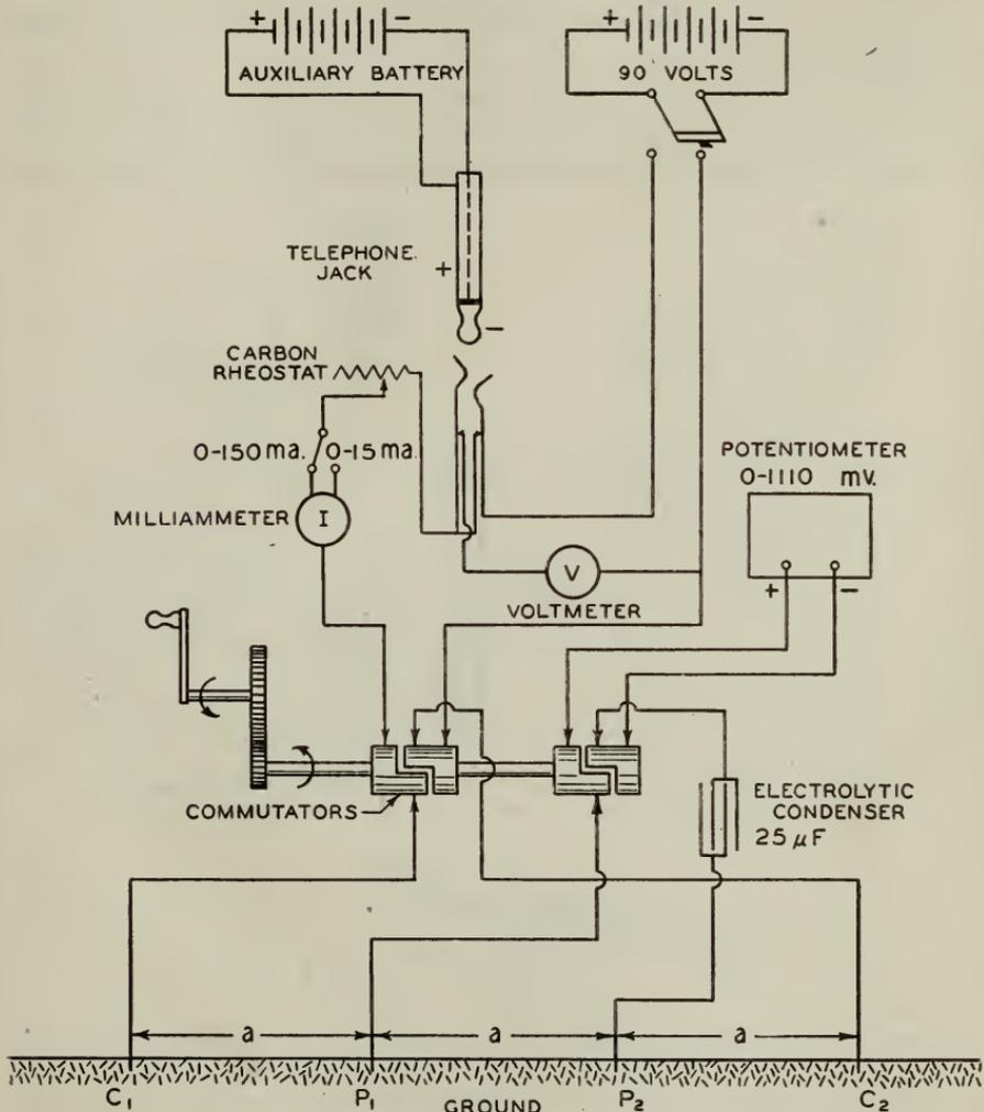
FIGURE 30.—Wiring diagram of the earth-resistivity instrument.
