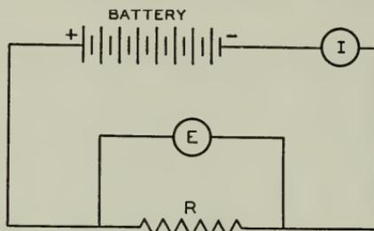
FIGURE 23.—Electrical circuit for measuring the resistance  $R$ .
