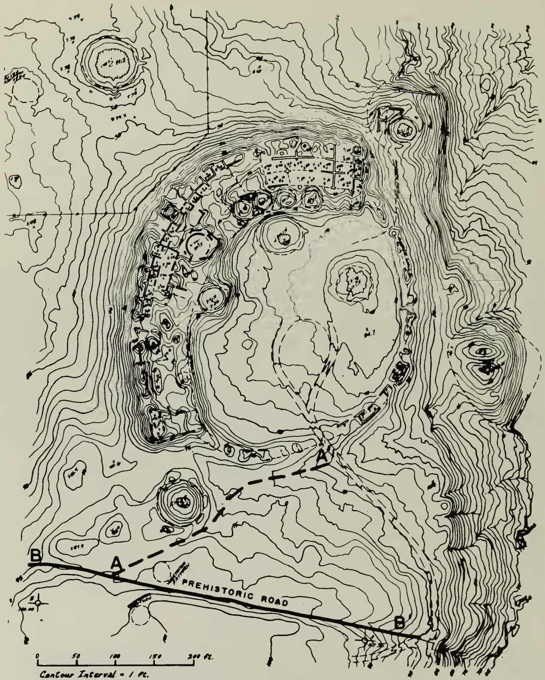
FIGURE 5 - Photogrammetric topographic map of Penasco Blanco ruin. B-B', a known prehistoric road; A-A', a prehistoric road inferred from contours.
