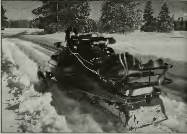
Figure 2. The study took place on flat terrain in Grand Teton National Park and involved a test snowmobile equipped for airflow measurement and exhaust sampling.
