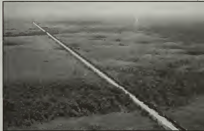
Figure 3. Built in the 1920s, the two-lane Tamiami Trail interrupts the natural north-south flow of water through Big Cypress National Preserve and Everglades National Park. Improving the conveyance of sheetflow through the highway is a critical aspect of ecological restoration in the preserve.
