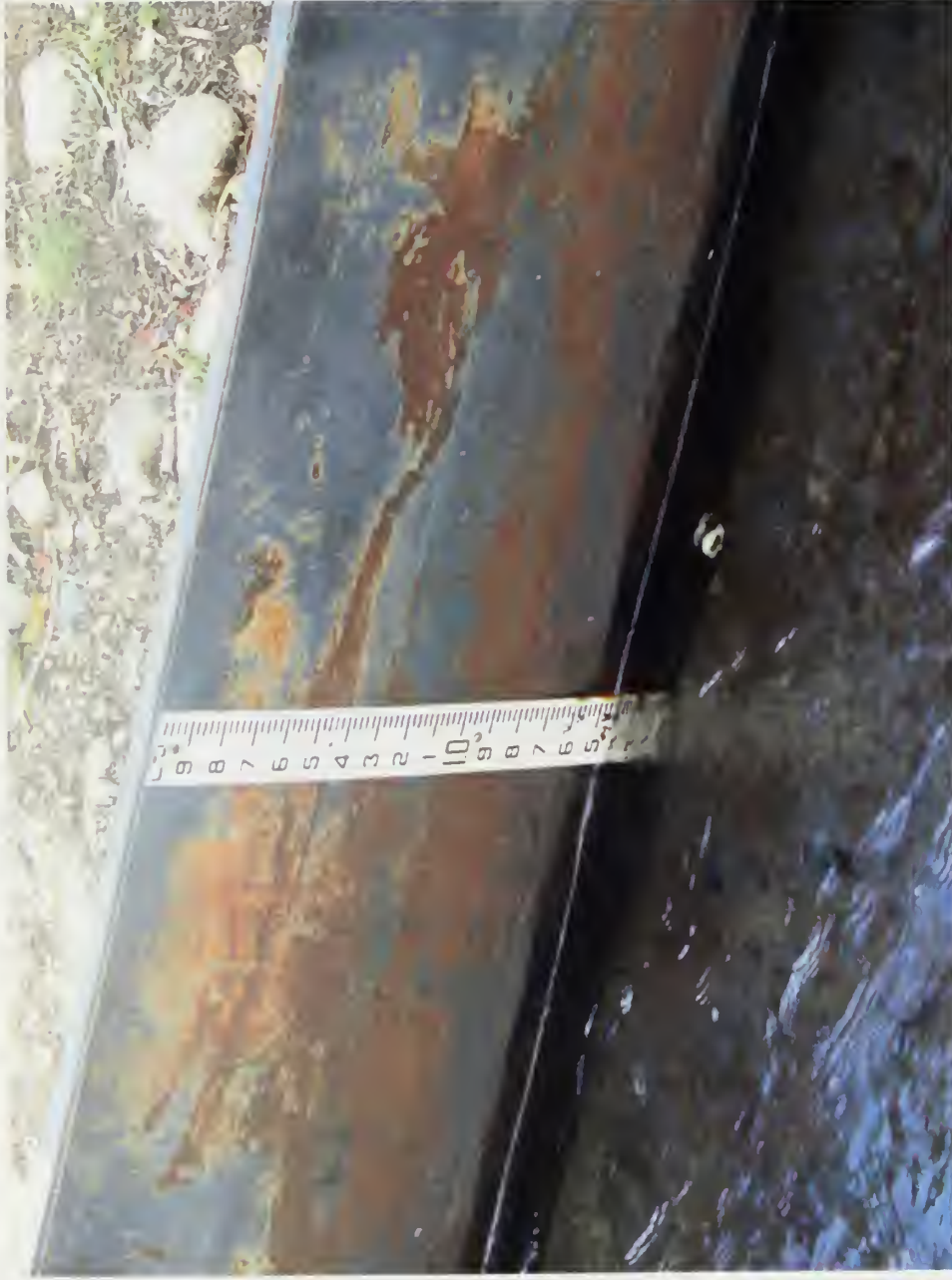
Cross Section: Deadman Creek #2.09.21.04_424 Deadman Creek at the Colorado Division of Water Resources flume. Staff gage bolted to the left bank upstream wall of the flume.
