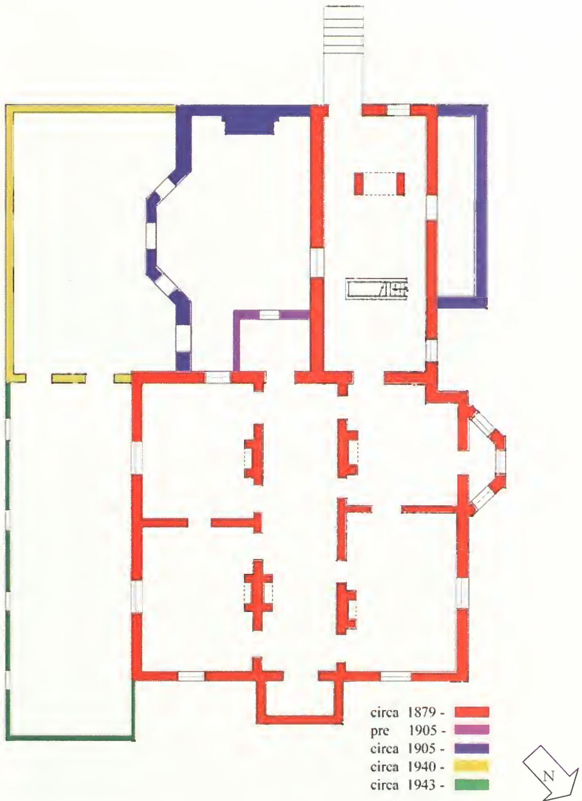
Figure 55. Officers Club, basement plan illustrating original appearance and alterations (not to scale).
