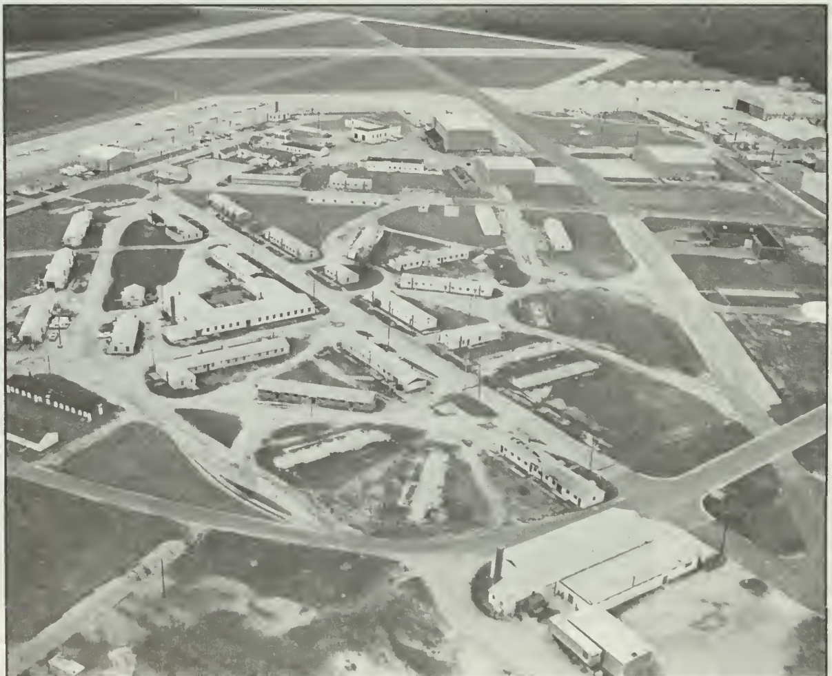
Figure 97. Millville Army Airfield, built 1941-42. As seen today, the complex of narrow, one-story concrete-block barracks are plain; hangars of corrugated metal are still used. Wettstein, 1990.
