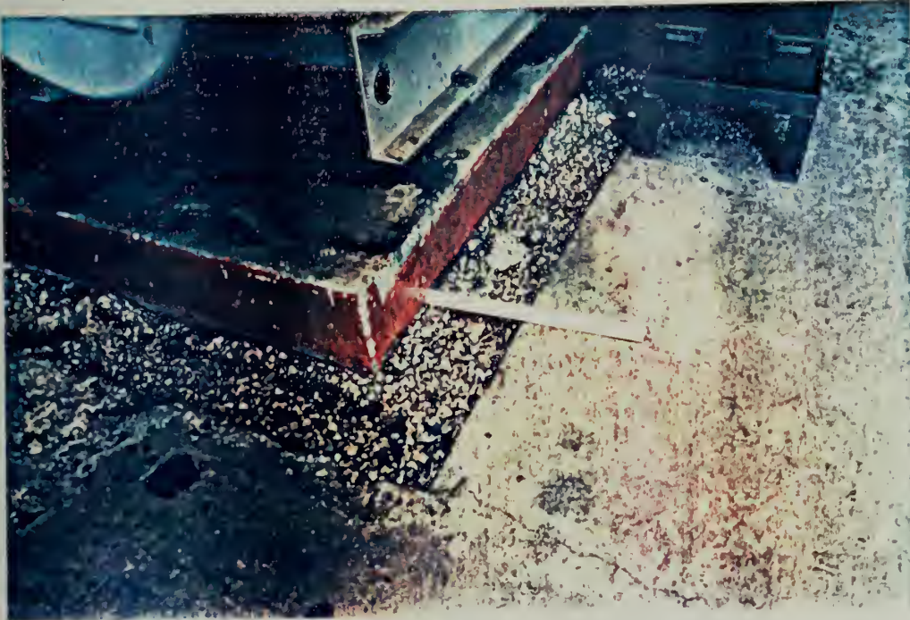
SAND BED FOR VIBRATION ISOLATION
