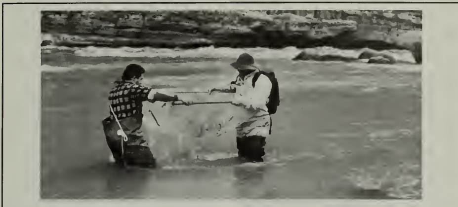
Samples collected by wading used the DH-81 Sampler
