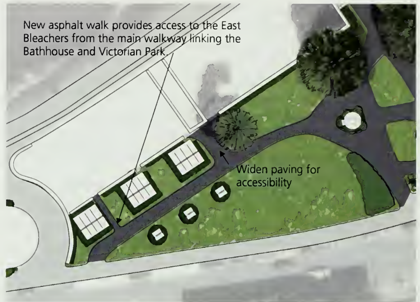
Figure 105. Plan view showing the areas behind the East Bleachers. (NPS, 2007)
