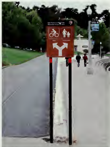
Figure 126. Placed at a height that allows cyclists to see it, this sign clearly denotes directional information as a way to reduce potential conflicts between bicycles and pedestrians, and is a useful model, compatible with standards for the NPS messaging system. (NPS, 2007)
