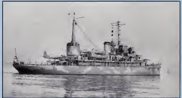
SMALL SEAPLANE TENDER (AVP) — Seaplane tenders featured a large crane to bring seaplanes aboard for servicing. An OS2U “Kingfisher” seaplane sits on the fantail of USS Barnegat (AVP-10) on New Year’s Day 1942. Many of the large group of small seaplane tenders built by the Navy during World War II became Coast Guard cutters after the war. BOSTS-10343
