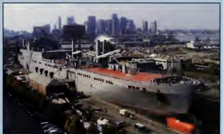
VEHICLE CARGO SHIP (AKR) — Vehicle cargo ships have boxy hulls to maximize internal vehicle storage and ramps to allow vehicles to be driven on and off. Named for Army Sgt. Cornelius H. Charlton, who received a posthumous Medal of Honor in the Korean War, USNS Charlton (T-AKR-314) is seen in Dry Dock 3 in Oct. 2003. Note the side loading ramp. Boston Ship Repair
