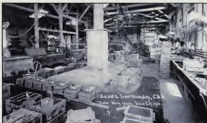
FOUNDRY, MOLD — A large number of molds can be seen in the foreground of this June 1901 view of the interior of the brass and iron foundry located in Building 16. These molds consist of frames containing wet sand formed around a pattern to create the cavity into which molten metal was poured. BOSTS-9279
