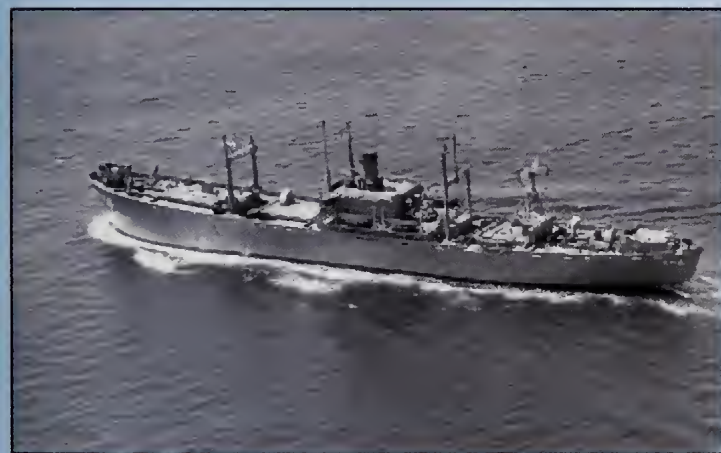
RADAR PICKET SHIP (YAGR; later AGR) — In the mid-1950s the Navy began to convert a series of “Liberty” ships into radar picket ships to supplement the land-based Distant Early Warning (DEW) network monitoring a potential Soviet air attack on North America. Naval Air Station Quonset Point took this aerial view of USS Searcher (YAGR-4) on May 29, 1956. BOSTS-14209
