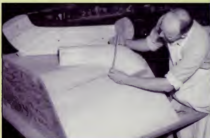
PATTERNMAKER — Patternmakers formed the wooden patterns from which molds were made for casting items in the Foundry.
