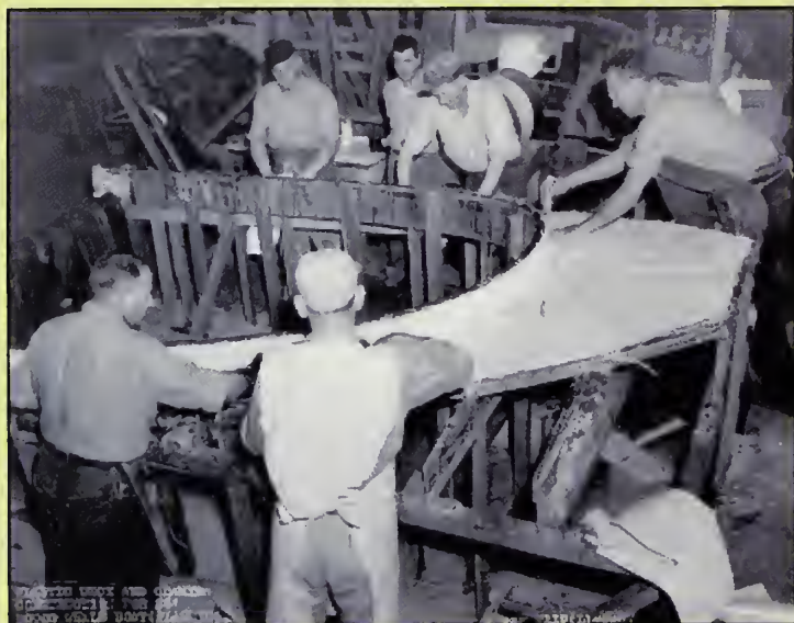
BOATBUILDER — The boatbuilder classification covered tasks involved in the construction of small boats. Here workers apply plastic (fiberglass) to a section of a 26-ft. motor whaleboat under construction in May 1957.
