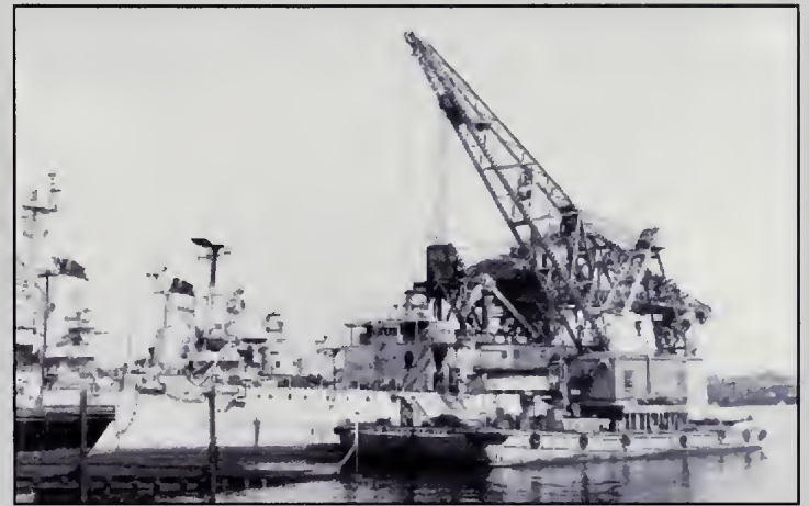
CRANE SHIP (AB)/FLOATING CRANE (YD) — Crane Ship No. 1 (AB-1) , converted from the battleship Kearsarge (BB-5) in 1920, was one of the best-known service craft assigned to the Navy Yard. She spent several periods at the yard, the last from 1948 until her sale for scrap in 1955. Shortly before her disposal, she is seen berthed with her replacement in the yard's inventory, the newly-delivered YD-196 . BOSTS-11624
