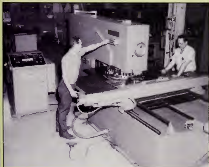
SHEETMETAL WORKER — Over time, technology automated many tasks previously done manually. This June 8, 1967, image shows Sheetmetal Workers Robert W. Benson (left) and Ernest Benedetto demonstrating the yard's new numerically controlled turret-punch press, which saved time by repeatedly and more precisely punching holes into metal plates. BOSTS-7732
