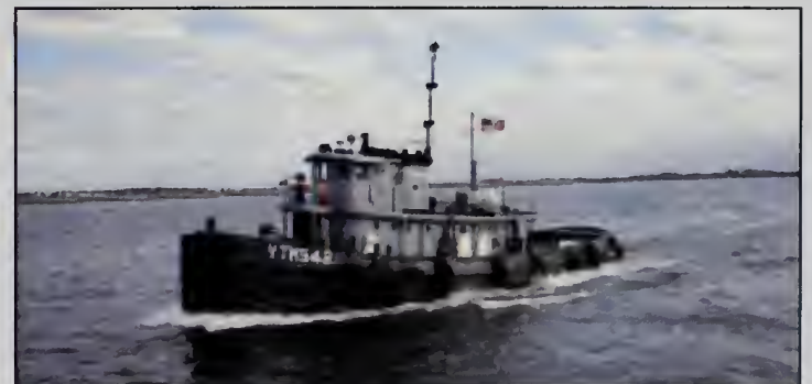
MEDIUM HARBOR TUG (YTM) — The harbor tug Chegodega (YTM-542) is seen on Nov. 10, 1972. Navy harbor tugs, used to maneuver ships into and out of docks and piers, were also equipped with firefighting equipment, as evidenced by the red nozzle forward of the pilot house. BOSTS-10680
