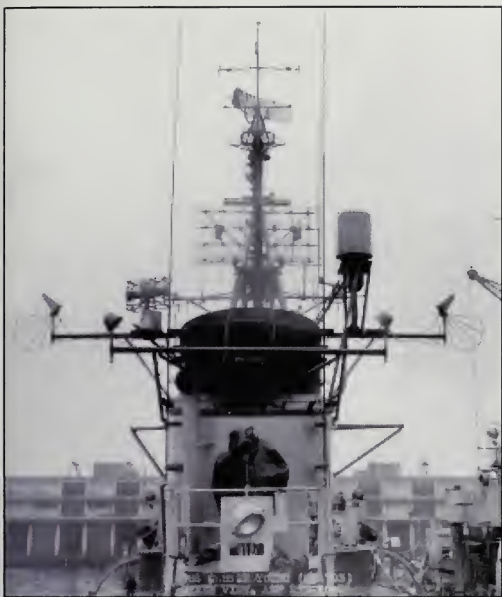
RADAR — Modern warships carry a large variety of radar antennas on their masts. This photograph, taken on Oct. 1, 1958, at the East Jetty of the South Boston Annex, shows the equipment mounted on the main mast and stack of USS Cassin Young (DD-793). BOSTC-1589
