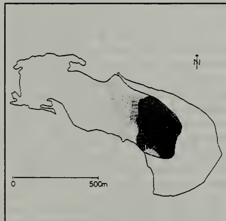
Figure 6. Digital map of snow water equivalence on the glacier surface. Snow was mapped using a binary regression tree with elevation and an avalanche index as independent variables. Lighter shades represent areas of greater snow accumulations; darker shades, shallower snowpack areas.
