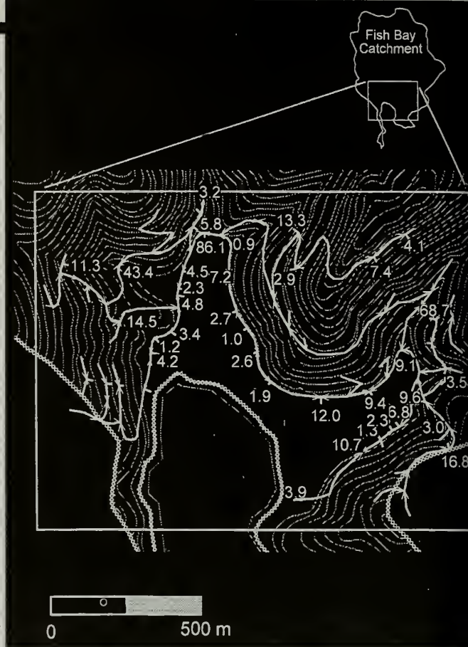
Figure 5. Road sediment delivery map of Fish Bay predicted by ROADMOD. Heavy lines represent the road network, dotted lines the elevation contours, and numeric values the road sediment delivery volume in cubic meters per year. Roads in the lower left part of the map are paved and have no sediment delivery values.
