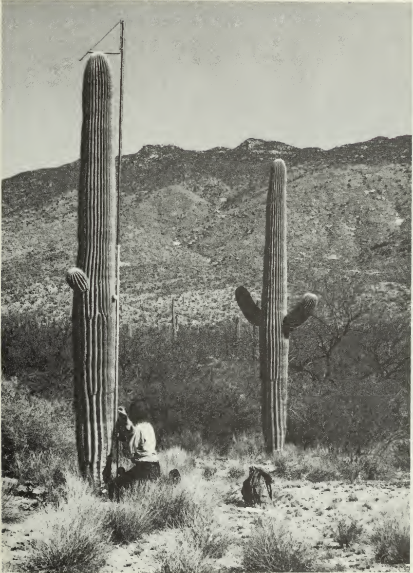
Fig. 37B. Height gauge used to measure apical growth of adult saguaros. Horizontal cross-bar rests on the tip of the plant. A steel measuring tape attached to the telescoping pole (vertically oriented with a spirit level) is used to measure the distance from the horizontal cross-bar to a permanent steel benchmark at the base of the saguaro. A meter-stick resting on the benchmark allows eye-level reading to the nearest whole millimeter. The apical growth increment is obtained by subtracting the previous measurement. Photographed 10 March 1974.
