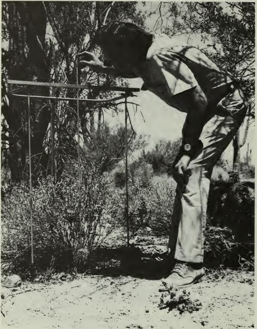
Fig. 37A. Height gauge used to measure apical growth of juvenile saguaros. Two aluminum legs that support the horizontal cross-bar rest on paired permanent benchmarks—steel rods set in concrete in the ground. The center measuring-rod rests on the stem tip of the young plant. The portion of the measuring-rod that projects above the horizontal crossbar is measured with a millimeter rule (measurement accuracy \pm 1 mm). Apical growth increment (week, month, year) is obtained by subtracting the previous measurement; center measuring-rod is placed in the same relative position on the stem tip for successive growth measurements. Using longer legs to support the cross-bar, the same method is used to measure young plants 1-2 m (3.6-6.6 ft) tall. Photographed 21 May 1972.
