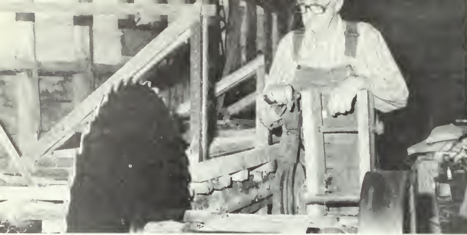
Elisha Payne cranks up his water-powered workshop, located at his mountain home near Blairsville. He built the workshop from the ground up, using mostly junked mechanical parts and scrap lumber. A water wheel, turned by water from a nearby creek, powers a generator and other equipment.
