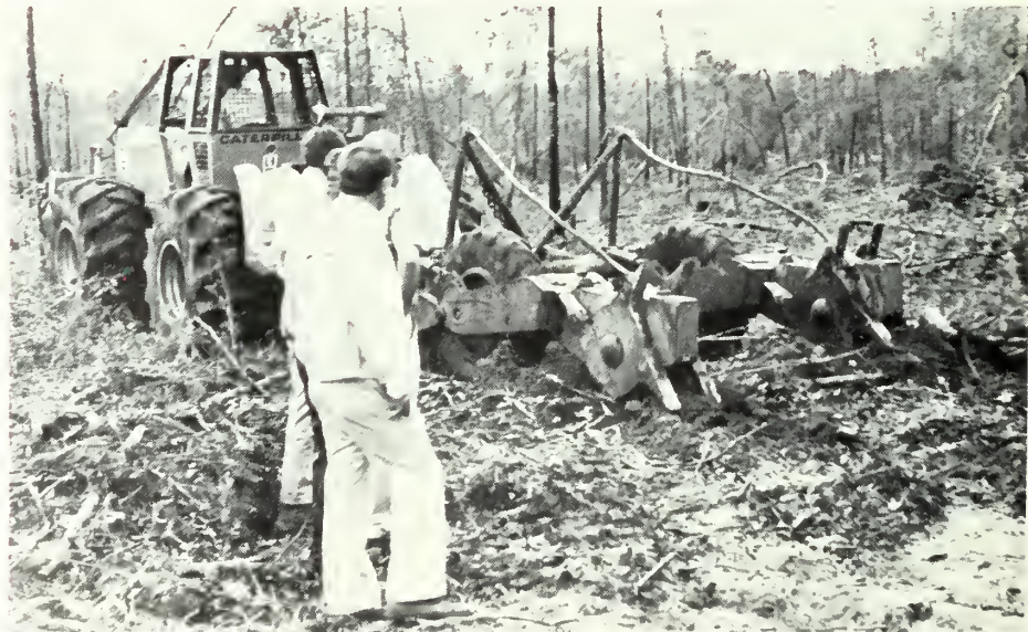
The Bracke Scarifier, a machine manufactured in Sweden which prepares the soil and plants forest tree seed as it moves across a field, is demonstrated by the Commission on a plot in Telfair County. The cost of the operation, an alternative to setting out seedlings, will probably run less than $40 per acre, according to foresters assigned to the study.
