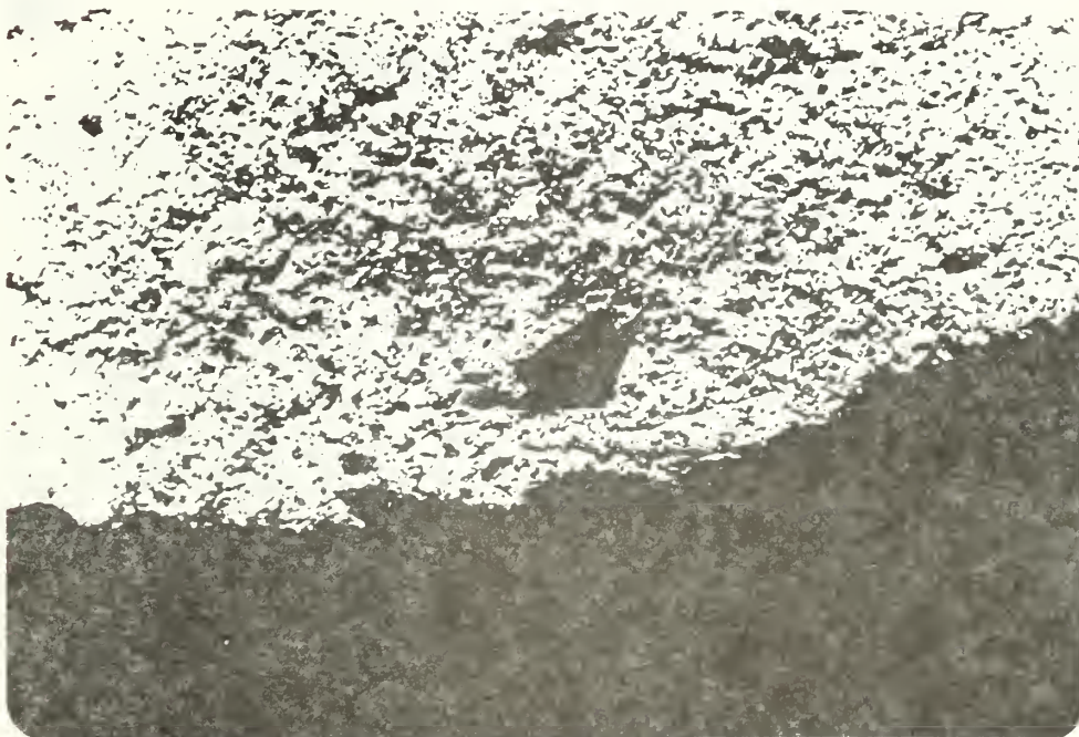
Figure 3: Detail of plaster Sample B showing edge fractures. Scale: approximately five times actual size.
