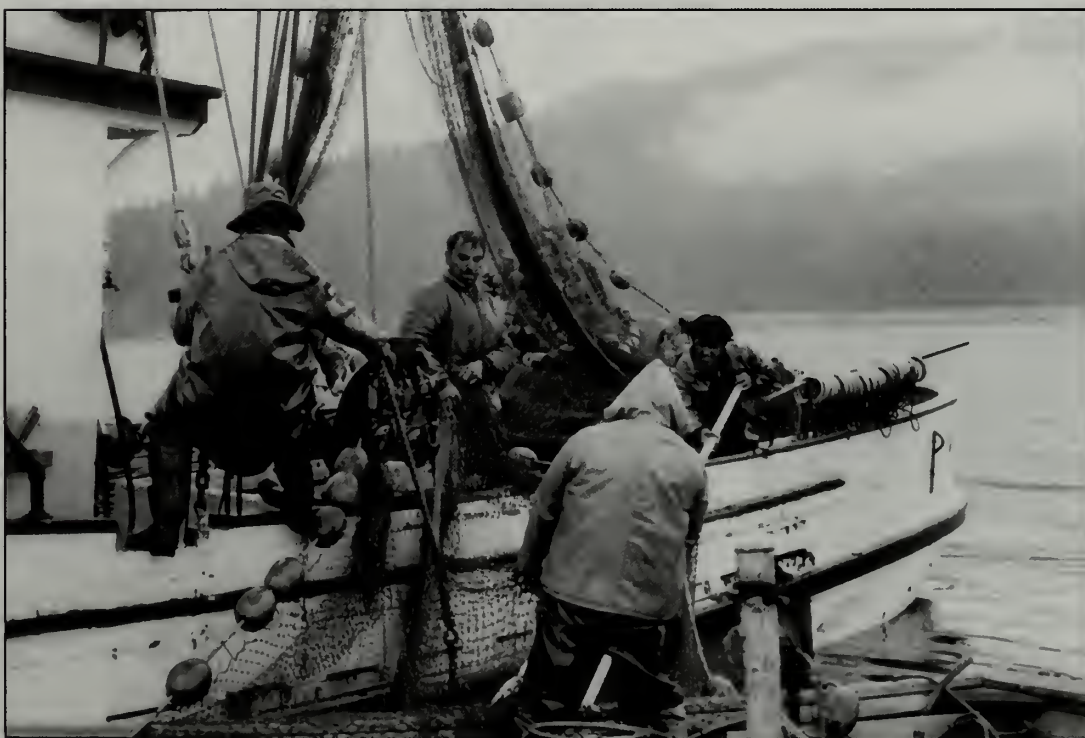
Figure 14: A crew hauls the net during "brailing." The "brailer" was a bag for transferring the fish from the seine to the hold. Each crewman had a station with specific duties. The man on the left is pulling the brailer line forward while the other two men – one on deck and one in the power skiff – are rolling the fish into the brailer. The man on the stern is shoving the brailer handle forward to scoop up the fish. Unseen is the "winchman" who coordinates with the "deckmen" pulling up on the brailer line until someone yells, "take 'er away!" Visible above the stern railing is the ring bar – an innovation that helped the crew organize different gear components around the deck. (Circa late 1950's-1960's, courtesy Huna Heritage Foundation)
