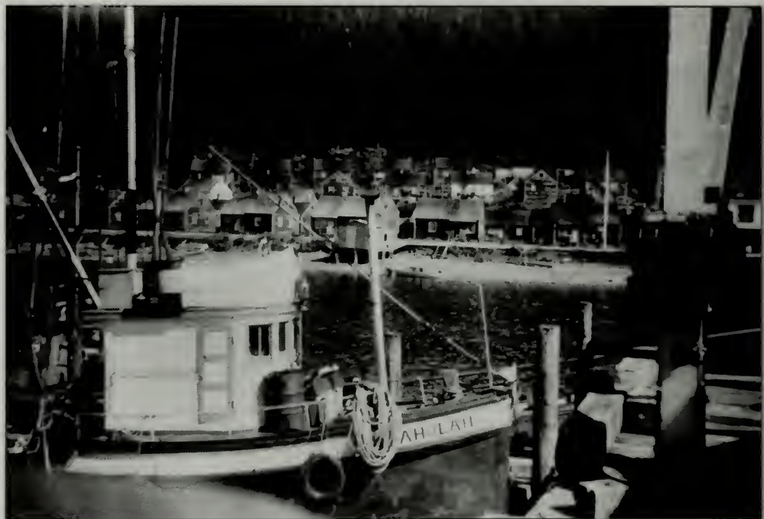
Figure 8: The FV Tahola , Captain John G. Fawcett, Sr., tied alongside the float at Kane's dock. The 55 gallon drum at the front of the cabin is fuel for the power skiff. The long stack in the bow is from the galley stove below. Many of the fishing boats during that time had their galleys forward in the forecabin (foc'sle). (Circa 1940-50's, courtesy Huna Heritage Foundation)
