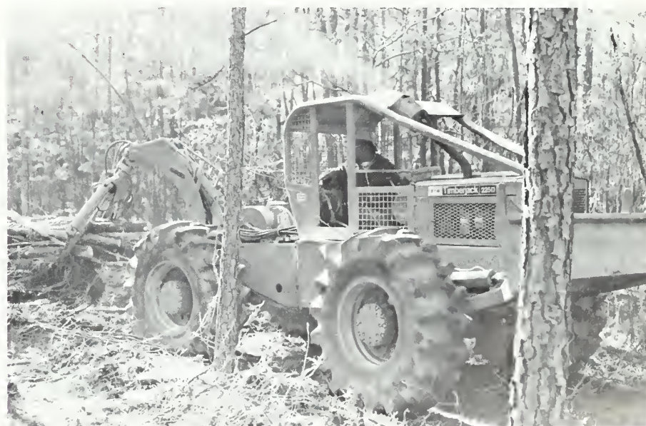
Grapple Skidder - Used to move felled trees to mechanical chipper.
