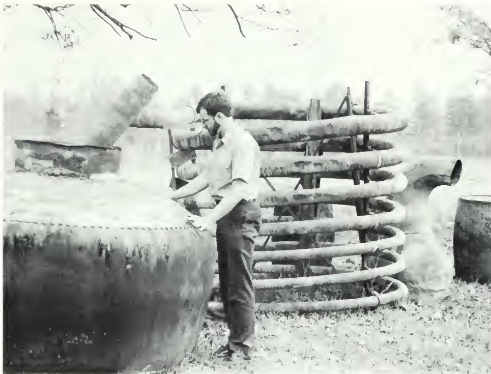
Forester Walker Rivers examines the giant condenser and boiler of the turpentine still to be restored and placed on display in the Georgia Forestry Museum.
