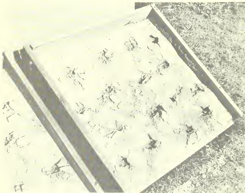
Figure 1.--Fill slope treatment of surface holes on dry, crusted surfaces.
