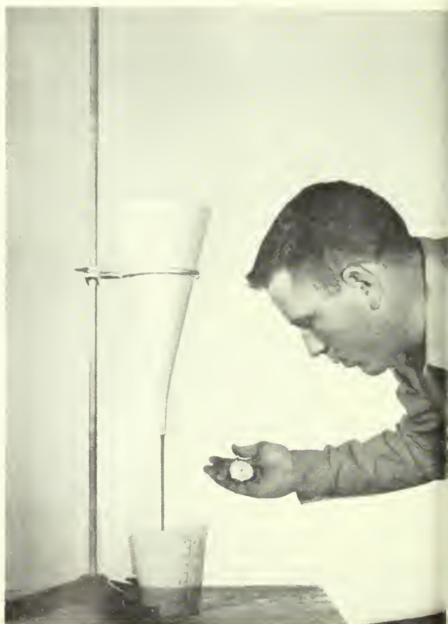
Figure 2.--Measuring viscosity with modified Marsh Funnel.
