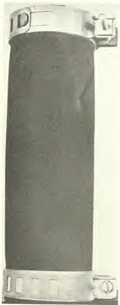
FIGURE 6.—RUBBER SLEEVE AND CLAMPS USED TO ENCASE SAMPLES FOR STABILOMETER TESTS.
