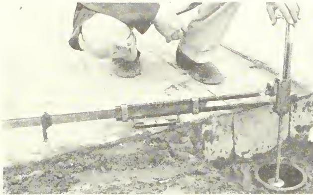
FIGURE 18.—DEVICE USED FOR MEASURING MOVEMENTS AT ENDS OF SLABS, AND BENCH MARK (LOWER RIGHT).
