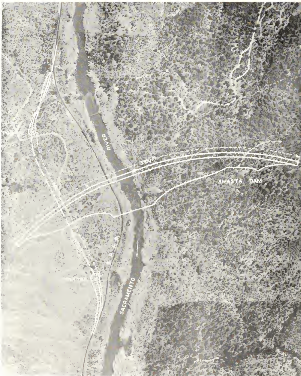
Aerial mosaic of dam site with dam and Southern Pacific Railroad bypass tunnel location indicated.
