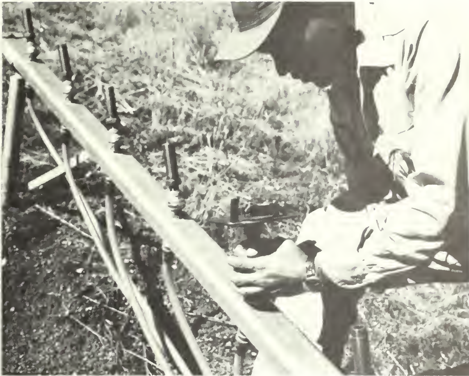
Figure 13.--One of the applicator nozzle racks showing hoses from pressure tank, flexible nozzle bases, type-F nozzles, and nozzle adjusting level. When setting the nozzle it is important to grasp the nozzle and not the level.
