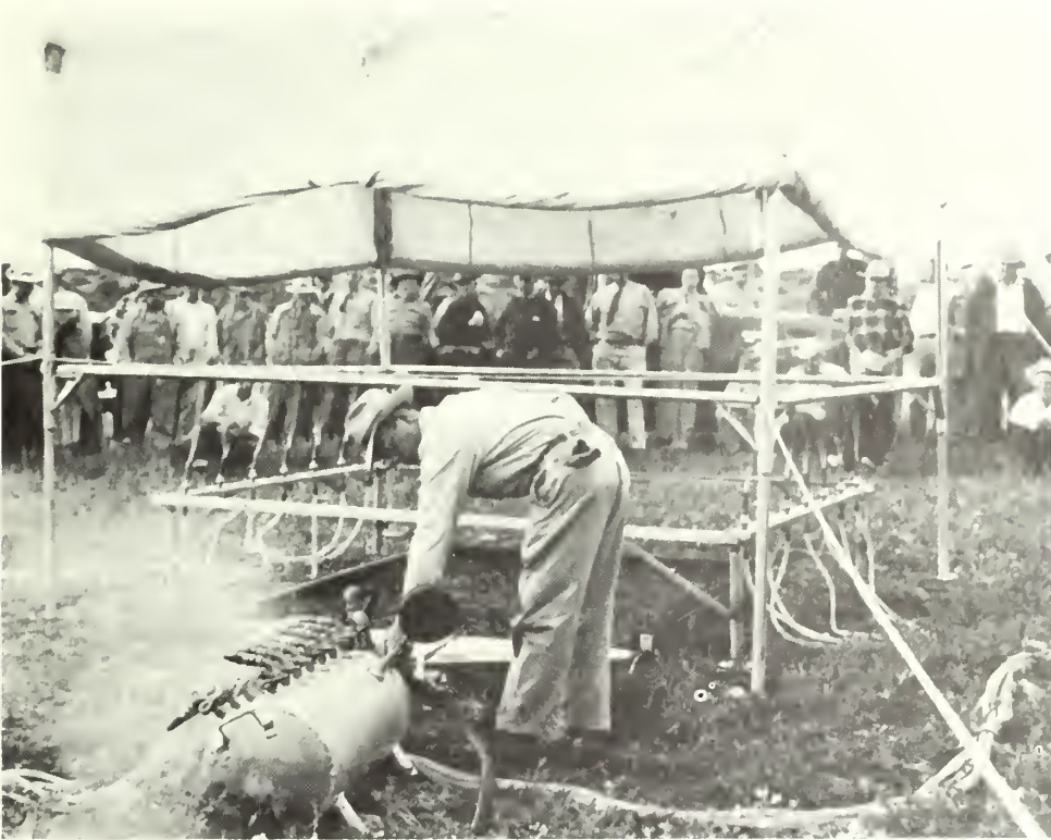
Figure 9--Demonstration setup of infiltrometer showing tent framework and cover. During normal tests, the cover is lowered for protection against wind disturbance.
