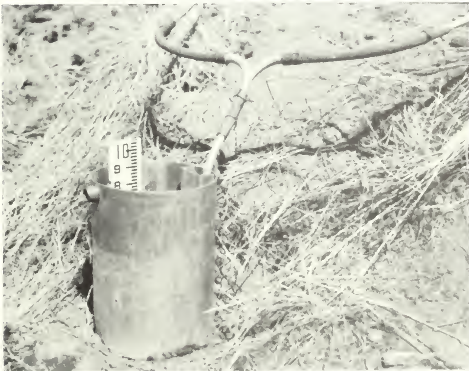
Figure 12.--Rainfall measuring can showing collector tubes from gages and porcelain staff gage.
