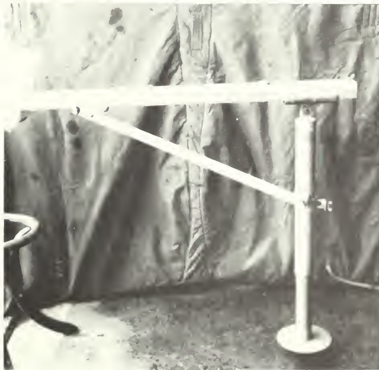
Figure 17.--Detail of rainfall applicator nozzle rack showing bushings for nozzles, tap and wing-nut for spreader bar, and leg assembly.
