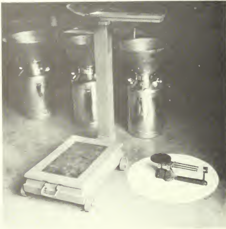
Figure 16.--Weighing cans, filter funnels, and platform scales for handling total discharge measurements and triple-beam balance for weighing discharge rate samples.
