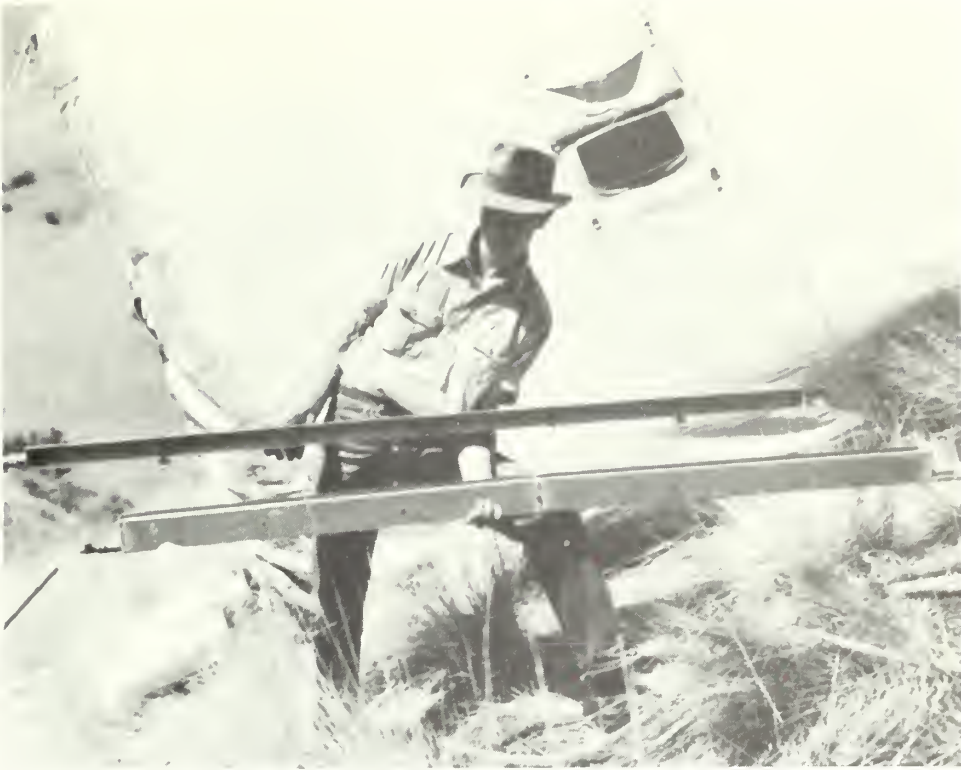
Figure 11.--Trough rain gages showing metal brackets for attaching gages to plot walls.
